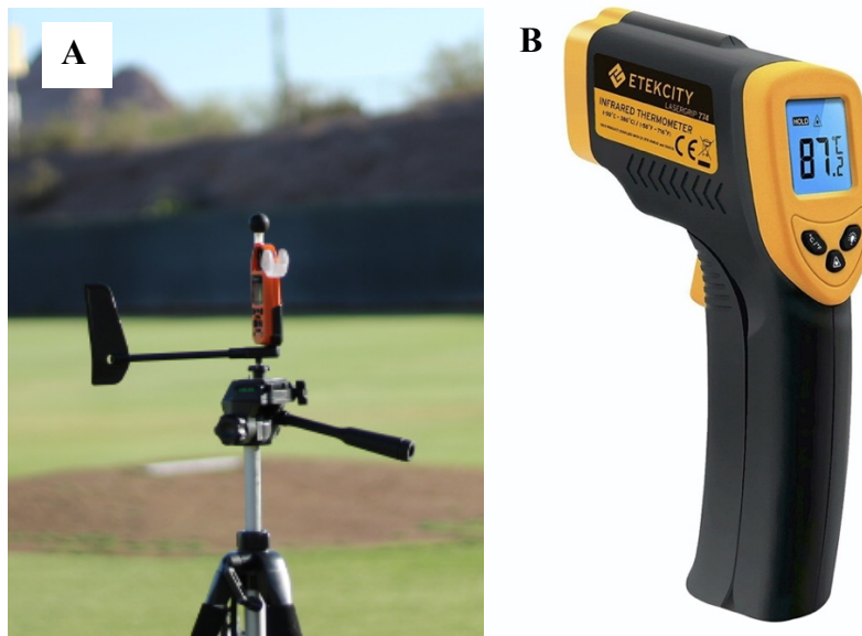
Photo 1: (A) the Kestrel 5400 Heat Stress Tracker during data collection (Photo credit: Jamie Teran, and (B) the Etekcity Lasergrip 774 Infrared thermometer from the etekcity website (“Etekcity,” n.d.).
