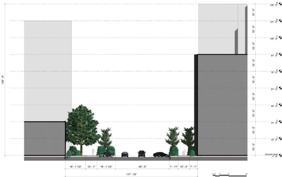
Figure 3. 3. Section view of the case study, E Tylor St and N 1st St in ASU Phoenix downtown Campus, Arizona.
