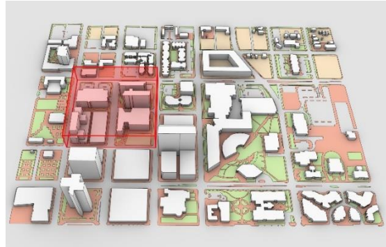
Figure. 4. 3. Rhino 3D model for The City of Phoenix downtown, with exact dimensions and heights from an official CAD drawings ASU facility management.
