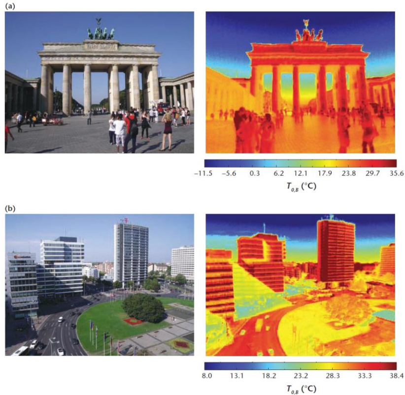
Figure. 2. 9. Visible and infrared (thermal) images for two urban landscapes in Berlin, Germany illustrating the radiation environment (Oke et al., 2017).
