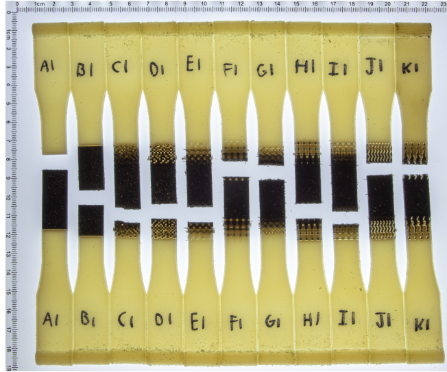
Figure 6.2: Failure Points for Samples with Centered Transition Regions
