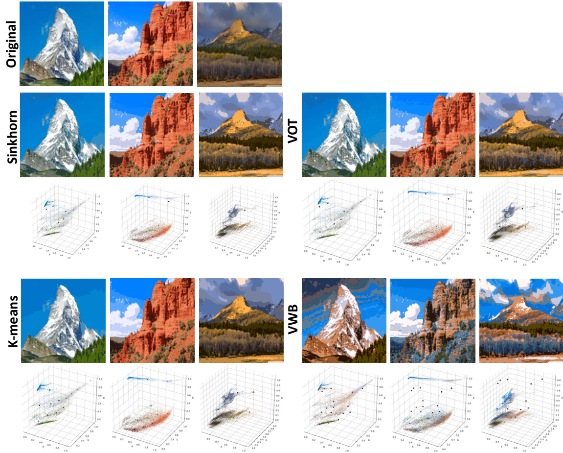
Figure 4.10: Quantizing RGB Values From 24 Bits to 4 Bits by Solving K-Means, OT, and the WB. Solving OT Results in Smoother Images; Solving WBs Can Cluster and Merge Colors at the Same Time.
