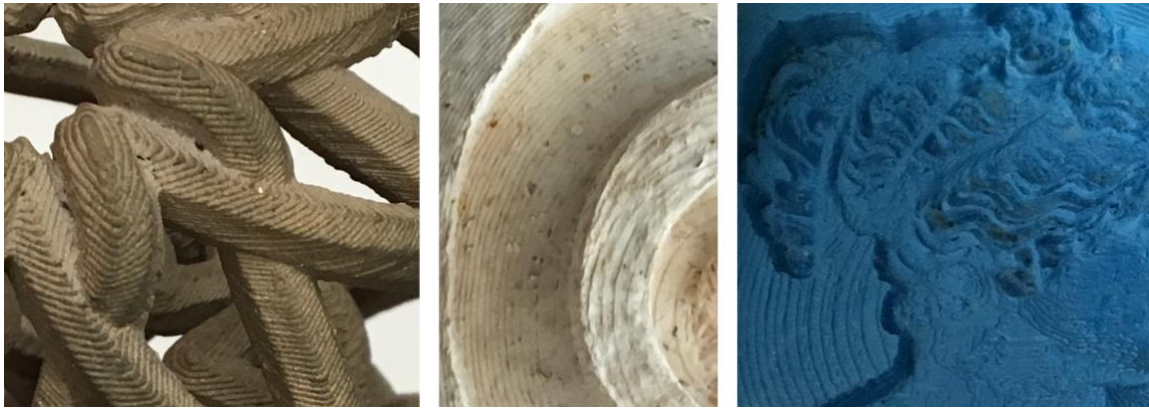
Figure 5.8 Print lines in objects created from 3D-printed designs. From left to right: cast bronze sculpture; mycelium object grown in silicone mold; silicone mold.
