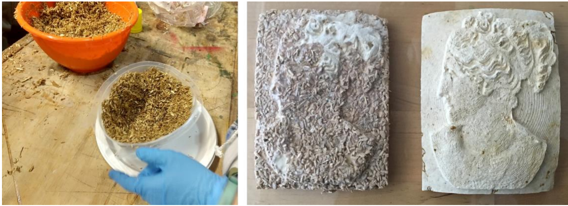
Figure 5.6 Biofabrication with mycelium. Left: mycelium spores mixed into an organic substrate. Right: mycelium objects shaped using silicone molds.
