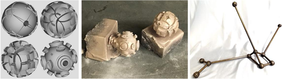
Figure 5.3 Process for creating a metal sculpture from 3D models. From left to right: 3D models; cast pieces; finished sculpture in which metal rods connect several 3D printed designs.
