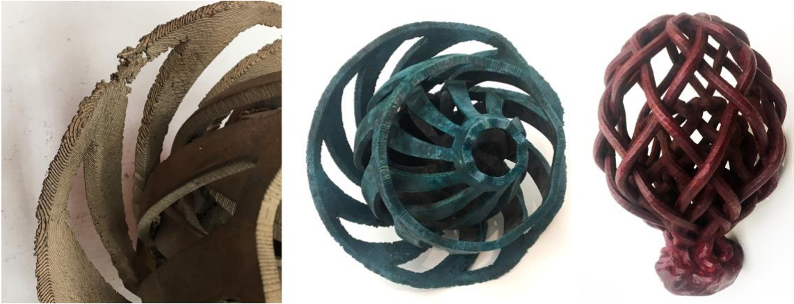
Figure 5.5 Bronze sculptures cast from 3D-printed designs. Left: detail of defect caused by metal casting process. Right: finished bronze sculptures with patinas
