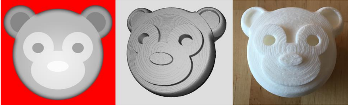
Figure 5.2 Workflow for generating 3D models from 2D images. From left to right: Source image; generated 3D model; 3D print.
