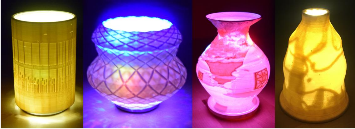
Figure 4.3 Examples of lithophanes created by participants with Lithobox. Custom images were mapped and extruded along the lithophanes' inner and outer surfaces, and each lithophane displays a unique image when lit from within
