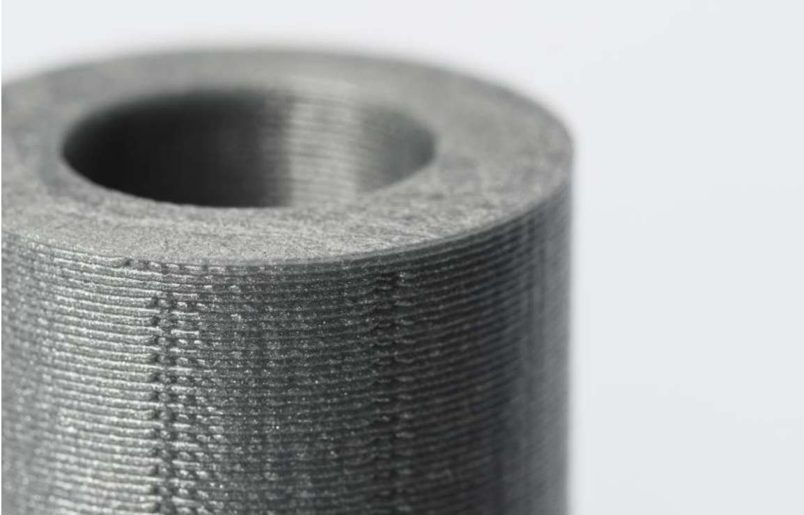
Figure 6.1. The Layer Lines of an FDM. these are Usually Visible [41].
