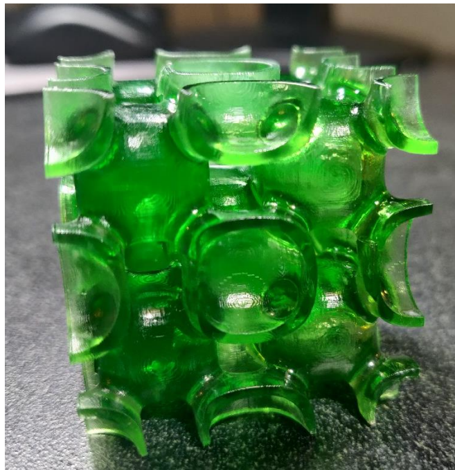
Figure 1.7. 40 x 40 x 40 mm 3-D Printed IWP Lattice Structure
