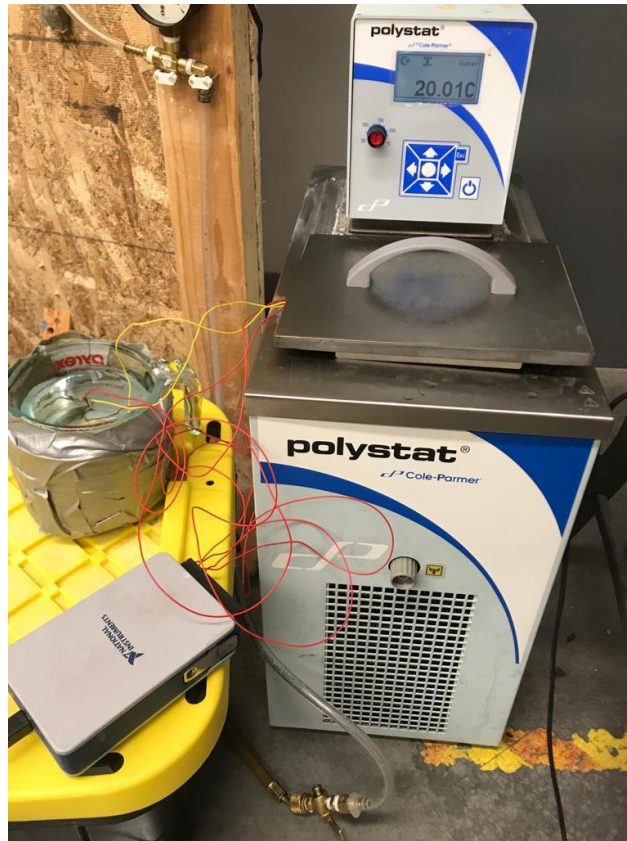
Figure 3.11. An image of the Thermocouple Calibration
