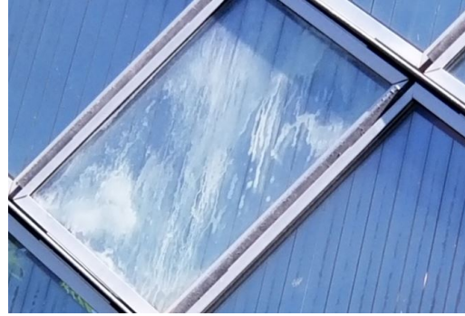
Figure 2.5: Closeup Showing Front Delamination of Solar Panel.
