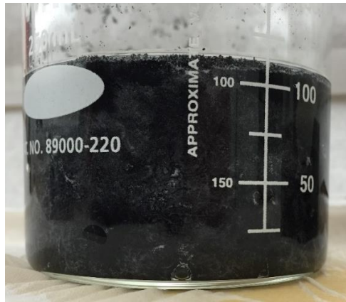
Figure 9 5% CNT/PEEK in Isopropyl Alcohol After Ultrasonic Mixing
