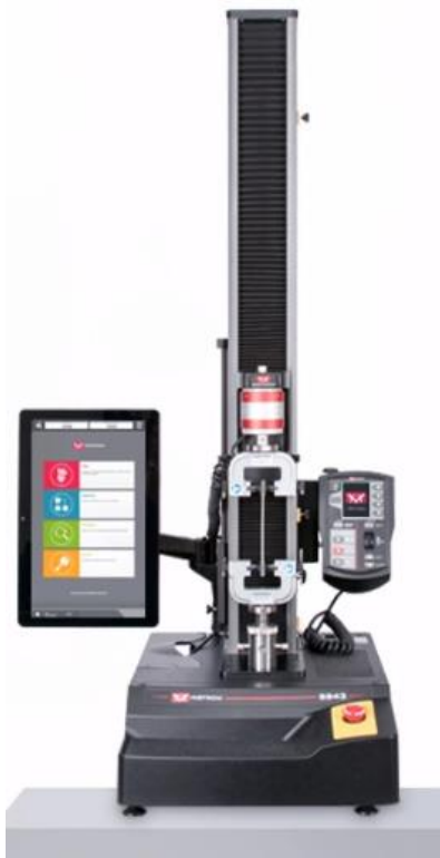
Figure 23 Instron 5944 Static Tensile Tester
