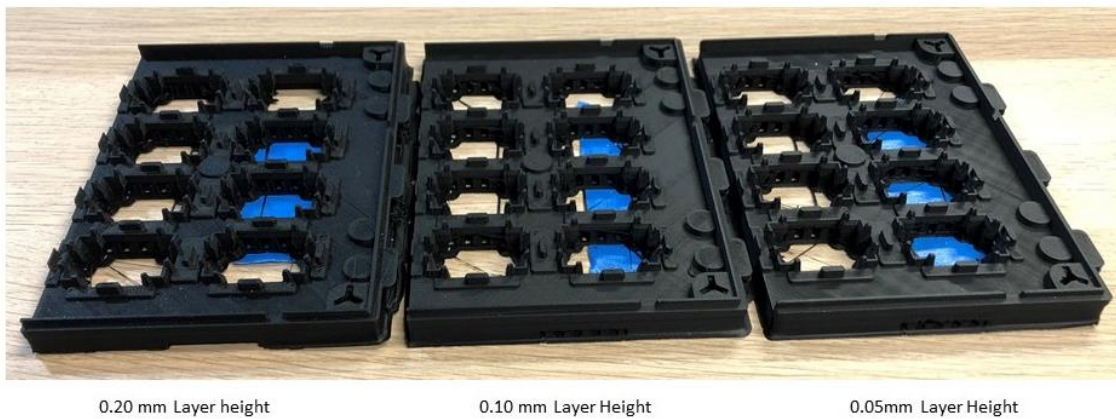
Figure 26 Trays Printed at Three Layer Heights
