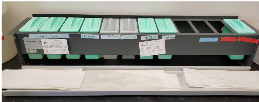
Figure 3.6.1. Tissue-Tek® Slide Holder and Rack. (a) Tissue-Tek® Slide Holder that can hold up to 24 slides (grey) and staining lid and dish. The grey rack fits inside the holder. Slides are fully immersed in liquid when 200 mL of fluid is in the container. (b) Tissue-Tek® Rack is a convenient way to organize multiple staining dishes used for deparaffinization and rehydration of tissue sections.
