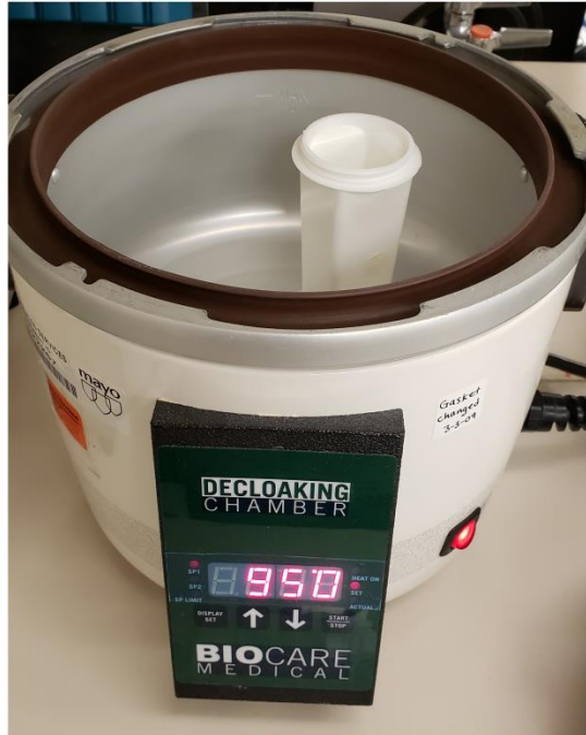
Figure 3.6.3. Decloaking Chamber (BioCare) with a Plastic Coplin Jar. Water (500 mL) is placed inside the decloaker to distribute the heat around the coplin jar.
