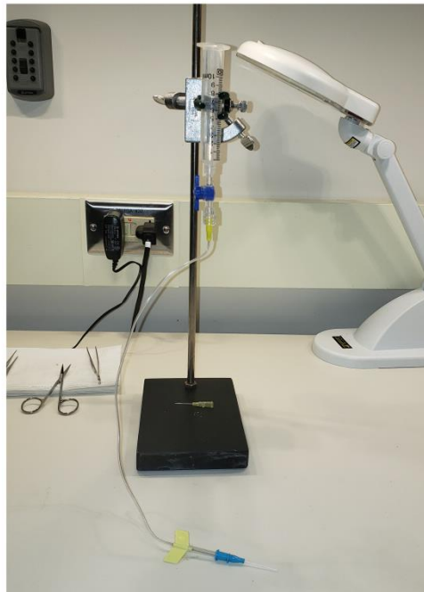
Figure 3.6.4. Syringe and Catheter Setup to Prepare Formalin Inflated Lungs. A 10-mL syringe is held in place by a clamp such that the 10-mL mark on the syringe is 20 cm above the benchtop. The blue stopcock controls the flow of formalin. The catheter is placed into the trachea during instillation of formalin.
