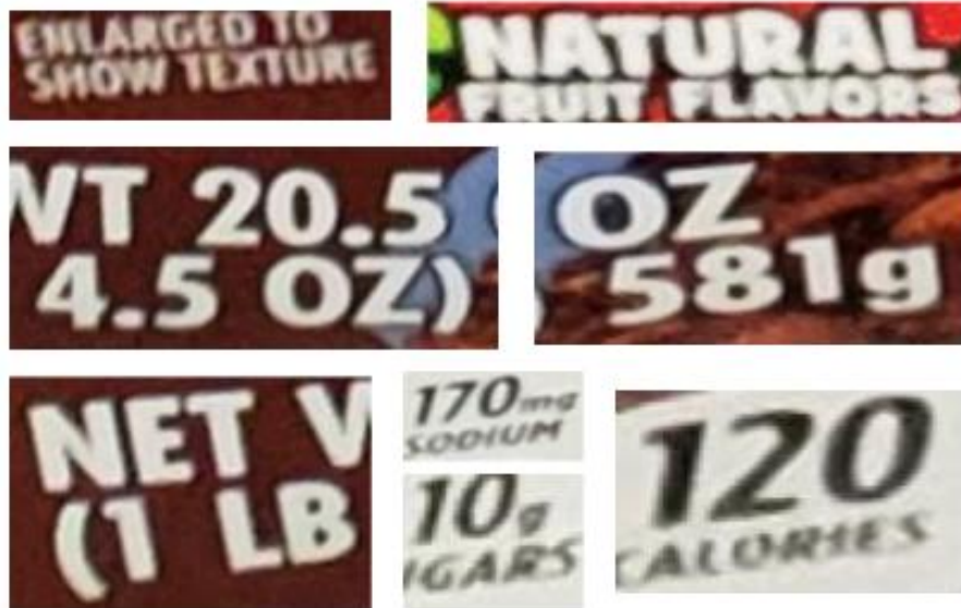
Figure 4.6: When using bounding box to crop the image segments, we extract more information than required. As seen in the above images, since it captures more text than required, it increases the probability of the text recognition model misclassifying the image segment
