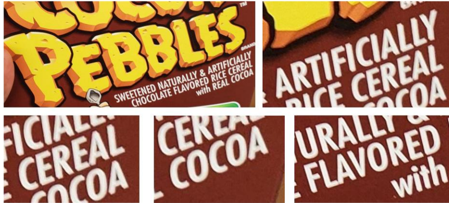
Figure 4.5: When using bounding box to crop the image segments, we extract more information than required. As seen in the above images, since it captures more text than required, it increases the probability of the text recognition model misclassifying the image segment
