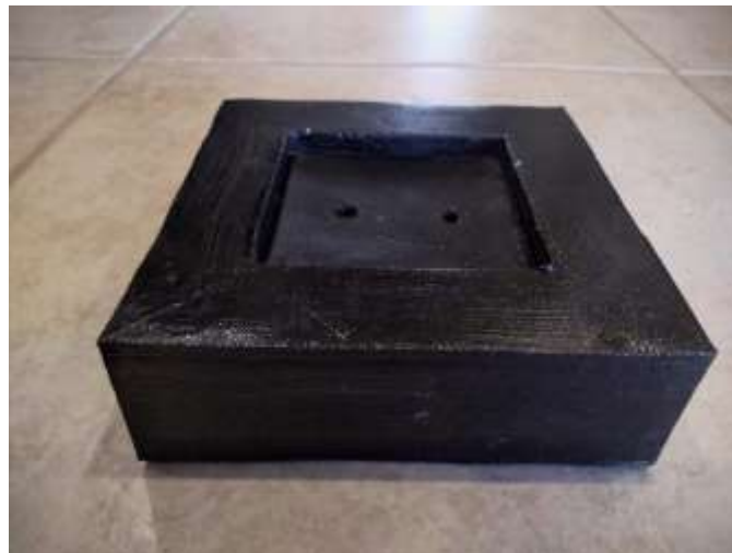
Figure 13: 3D printed Float that was Coated with Paint and a Waterproof Spray.
