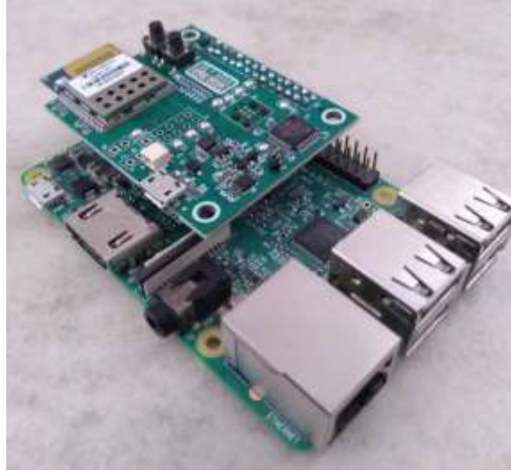
Figure 24: DMW1001 Module Circuit Board Connected to the Raspberry Pi 3 Model B+.
