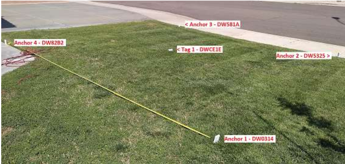
Figure 27: Second Test of the System Using the Raspberry Pi Outdoors with Anchors Labeled at 5m Away.
