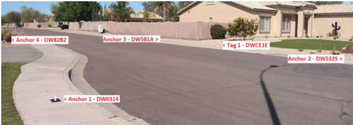
Figure 29: Third Test of the System Using the Raspberry Pi Outdoors with Anchors Labeled at 13.5 m Away.
