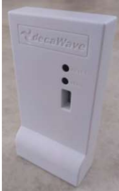
Figure 16: DMW101 Module Used as the Anchors and Trackers in the Location System.
