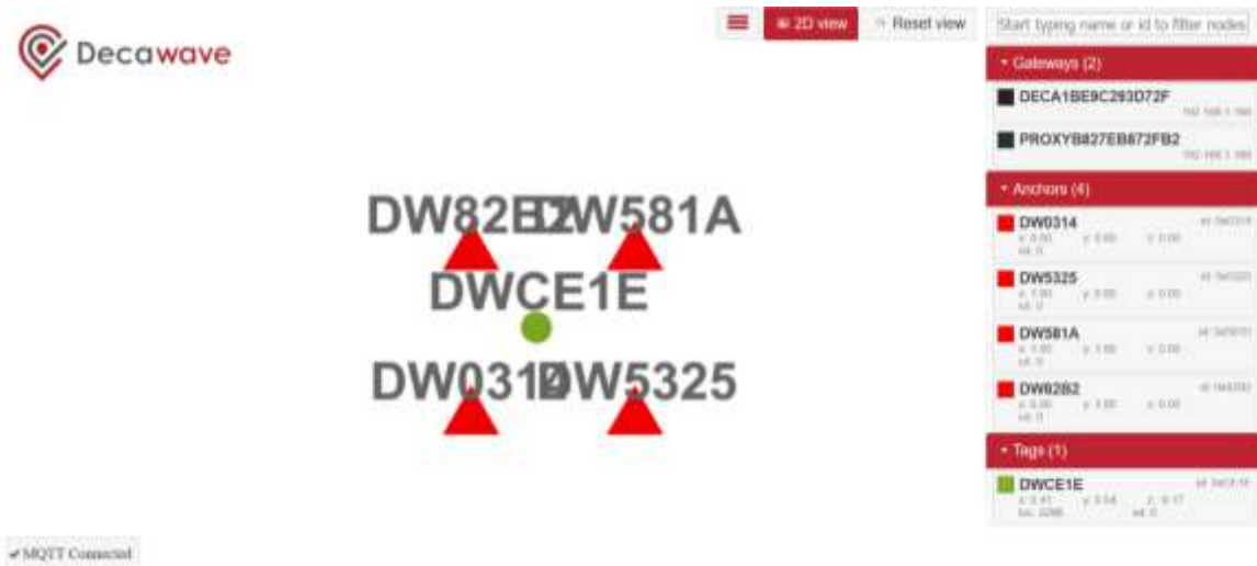
Figure 26: Network Page Displaying the Locations of the Anchors and Tag in the Initial Test.
