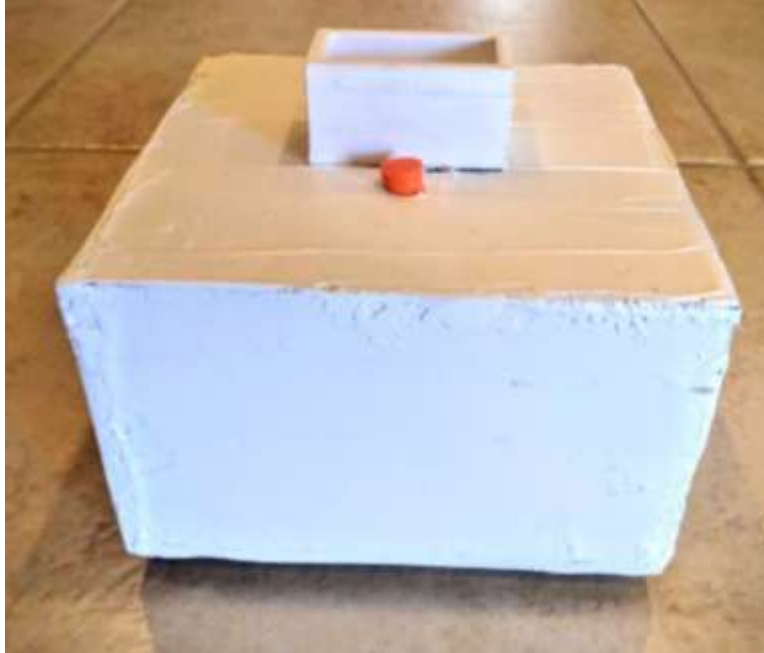
Figure 15: 3D Printed Float with Waterproof Sealant and Plug.
