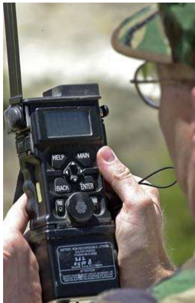
Figure 2: A Lt. Commander Using a Combat Survival Evader Locator (CSEL) During a Survivor Extraction Exercise. (Fallon Naval Air Station, 2001).
