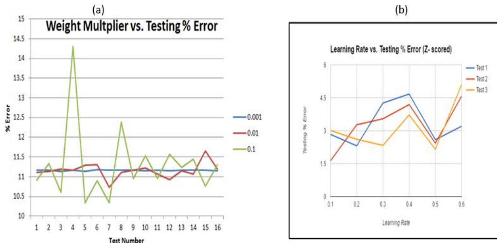
Figure 5. (a) The Effect of Weight Multiplier on the Error (b) The Effect of Learning Rate on the Error
