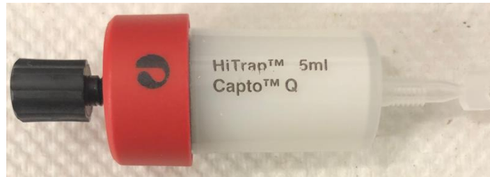
Figure 20. HiTrap CaptoQ Anion Exchange Column (GE Healthcare) Utilized for Purification
