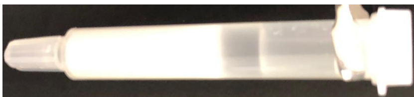
Figure 21. PD MiniTrap G-10 Desalting Column (GE Healthcare) Utilized for Buffer Exchanging Virus Sample.
