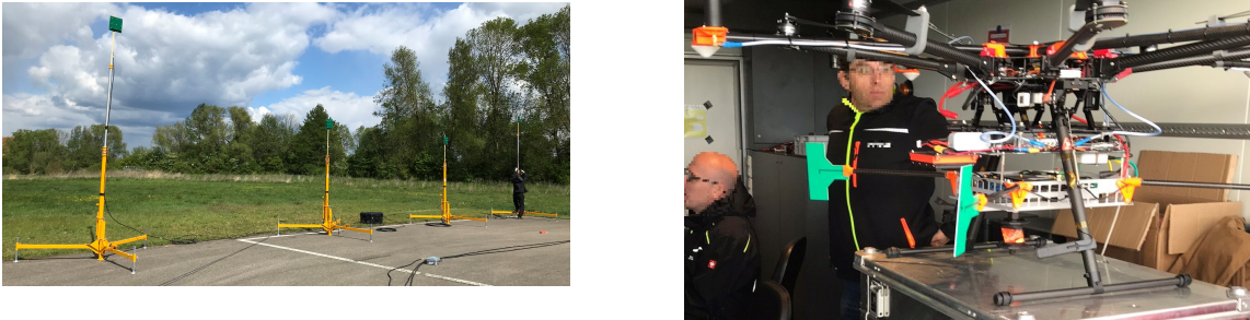
Figure 6.5: Experimental testbeds for the flight tests in Nördlingen, Germany. The base-station (left) consists of 4 antennas mounted on telescoping platforms. The hardware is mounted in the black box in the center of the picture. The UAS (right) is a DJI S1000+ UAV equipped with the hardware mounted in an aluminum frame and a tachymeter reference.
