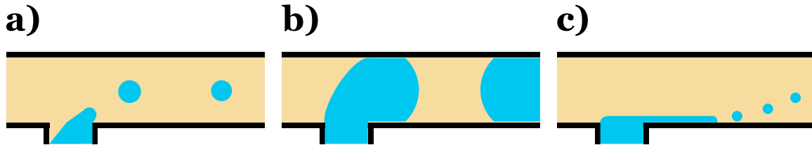
Figure 2.3 Illustrations of droplet breakup regimes. (a) dripping, (b) squeezing, and (c) jetting.
