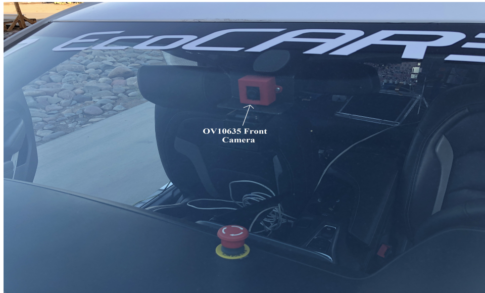
Figure 5.6: OV10635 Mounted on the Test Vehicle.
