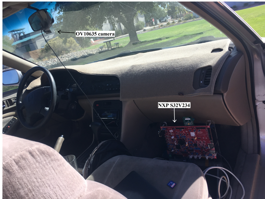
Figure 5.1: Test Setup to Capture Video Data.
