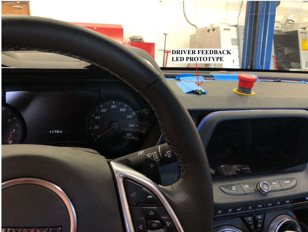
Figure 5.14: Driver Feedback LED Prototype. In This Setup, a Single LED Is Used to Test the Functionality.
