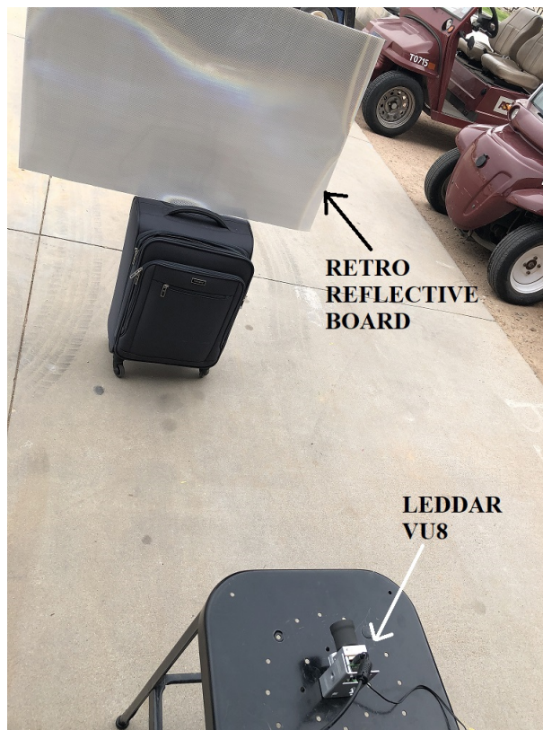
Figure 5.5: Leddar Vu8 Test Setup. Retro Reflective Board Used as Target to Test the Range of the Leddar Vu8 Sensor.
