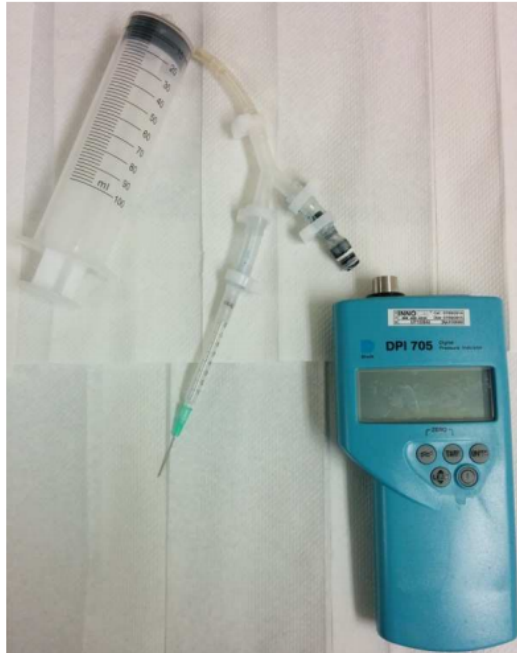
Figure S2.3. Depiction of leak and burst pressure testing device. Bifurcated tubing from a syringe leads to a digital manometer and a needle. The needle is inserted into clamped intestine and filled with saline solution. Simultaneously, the pressure is recorded when leakage first occurs from the intestine (leak pressure) and at the maximum pressure reached (burst pressure).
