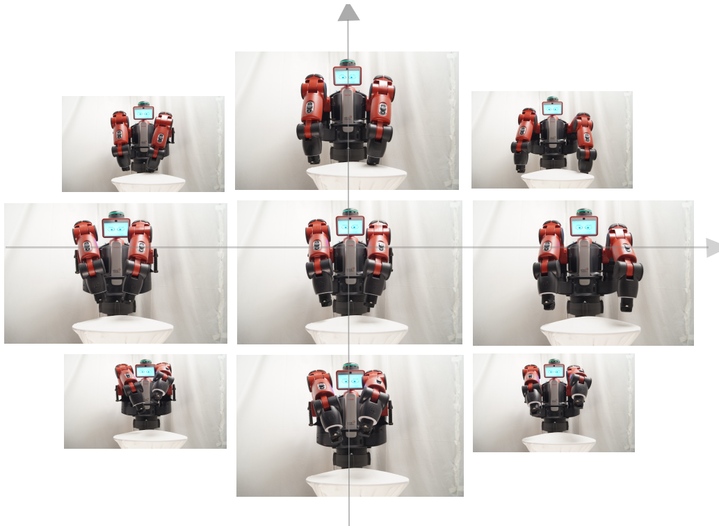
Figure 3.10: Two synergies and their combinations found during the execution of the GrouPS algorithm for learning to lift the orange ball. The horizontal axis is showing a synergy of closing and opening motions whereas the vertical axis represents a up-and downwards movement of both arms. Different combinations of those synergies are shown in the four corners of this figure.
