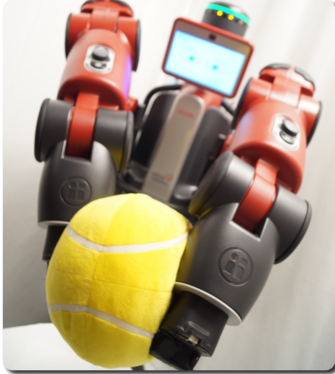
Figure 3.1: A bimanual robot learns to lift an object while simultaneously identifying synergies among the control variables.
