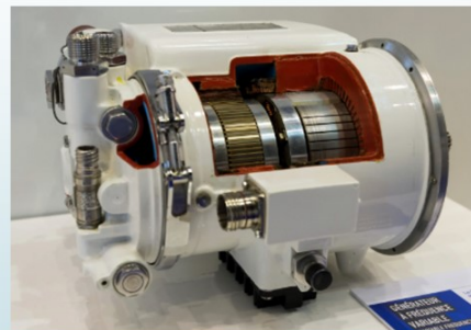
Main AC Generator
