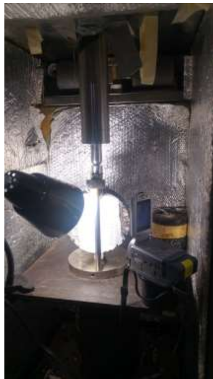
Figure 20. Typical C* Fracture Test Setup
