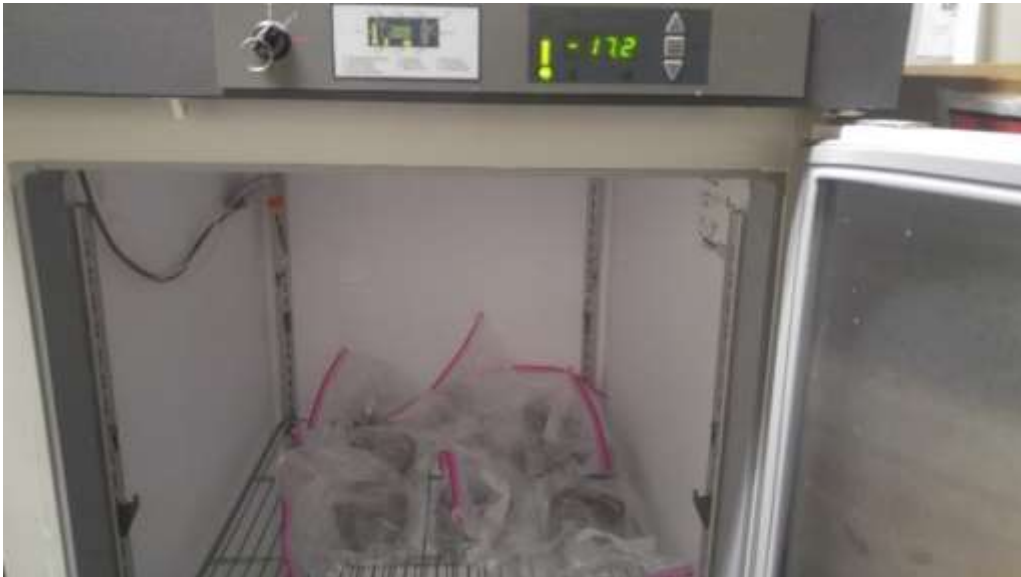
Figure 22. Specimens During the Freeze Cycle
