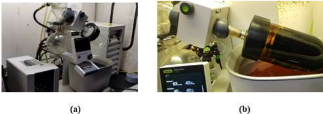
Figure 38. Binder Recovery using RotoVap (a) Equipment and (b) During Flask Immersion in the Hot Oil Bath
