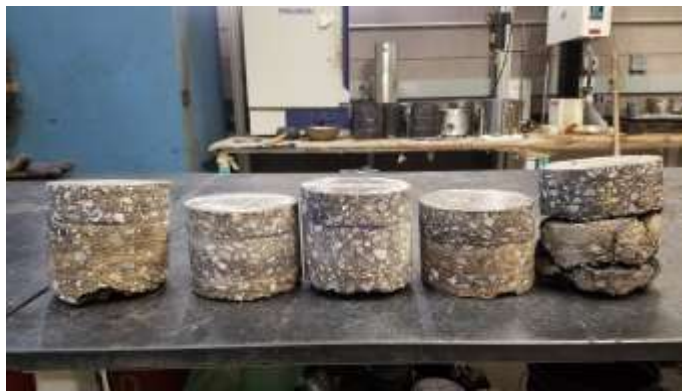
Figure 49. Cores Taken from 15% RAP Section
