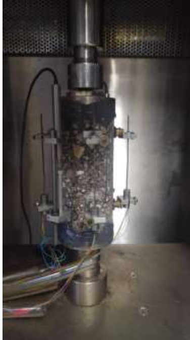
Figure 21. Uniaxial Fatigue Test Setup
