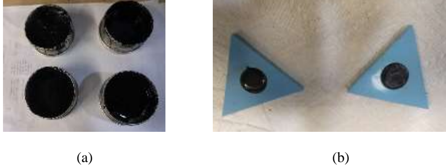
Figure 39. Recovered Binder Poured Into: (a) Metal Cans Then (b) DSR Specimen Molds
