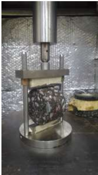
Figure 24. Specimen During IDT Testing
