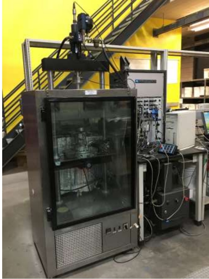
Figure 16. UTM Machine Used for Flow Number Testing
