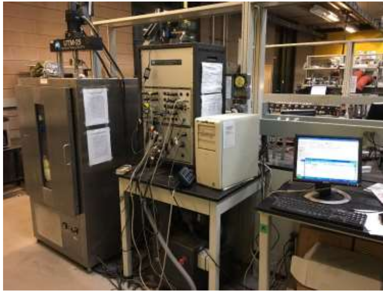
Figure 14. UTM Machine for Dynamic Modulus Testing
