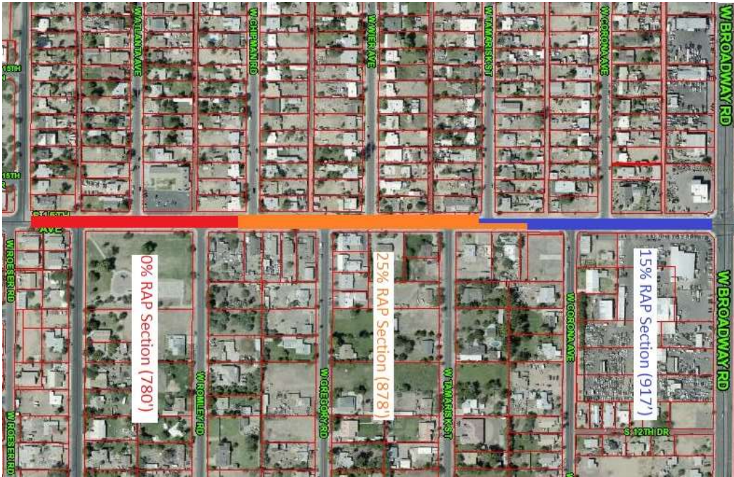
Figure 12. As-Constructed Map of the Sections
