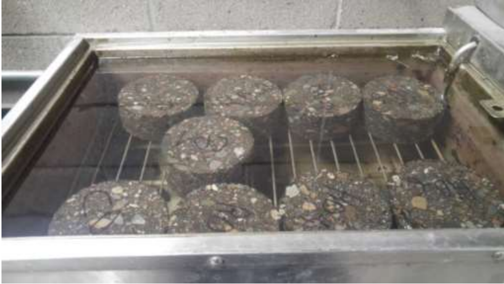
Figure 23. Specimens During the Thaw Cycle
