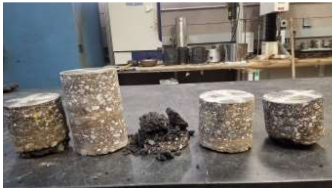
Figure 50. Cores Taken from 25% RAP Section
