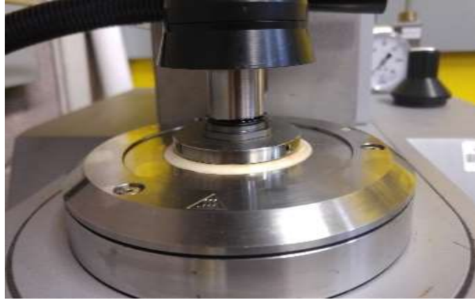
Figure 41. MSCR Test Setup
