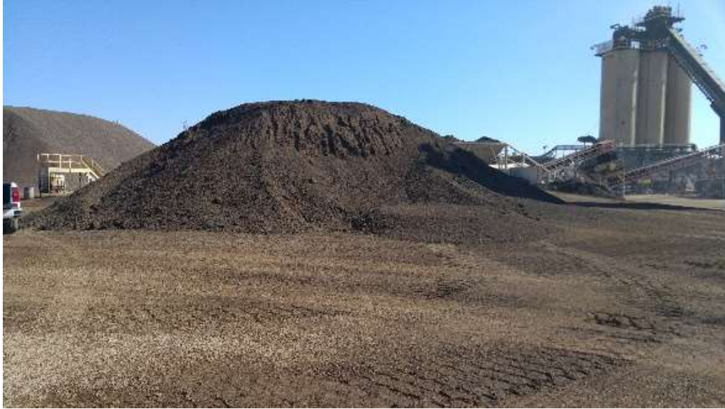
Figure 6. Processed RAP Stockpile
