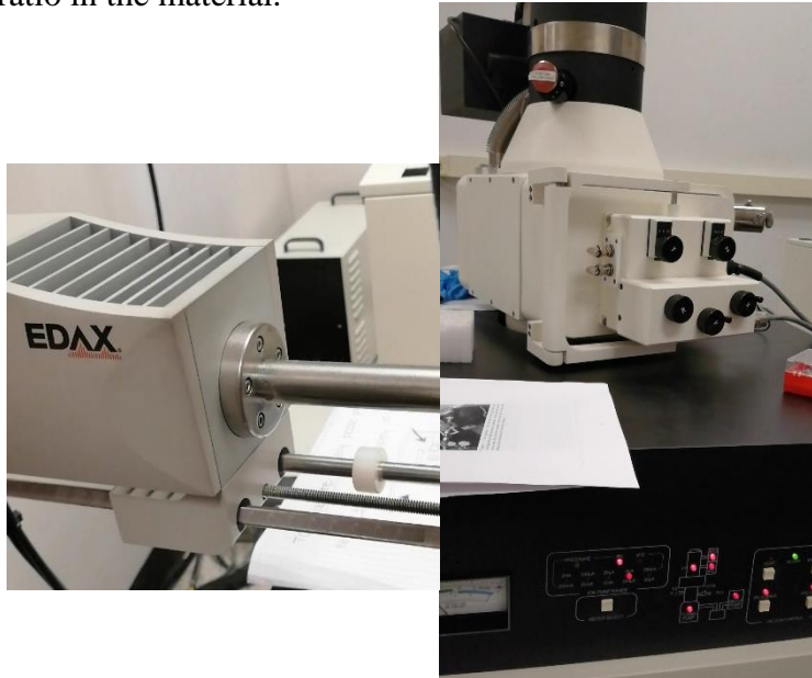
Figure 12. images of EDAX detector (left) and SEM (right). [26]
