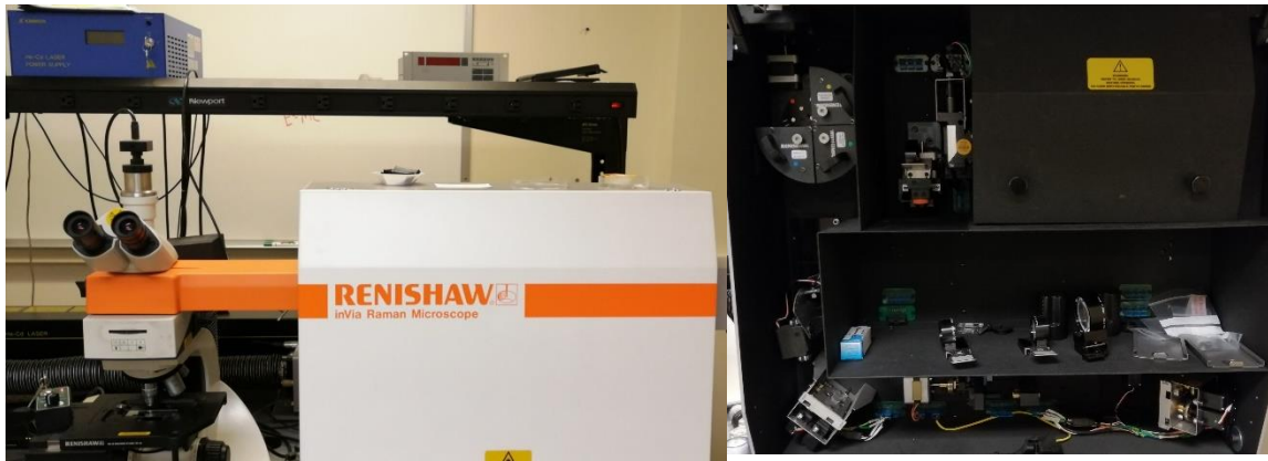
Figure 8. Raman Spectroscopy with light microscopy, blue laser, and UV laser source. On the right is inside the Raman with filters and lenses to increase emitted wavelength accuracy then read Raman scattered data. [F8]
