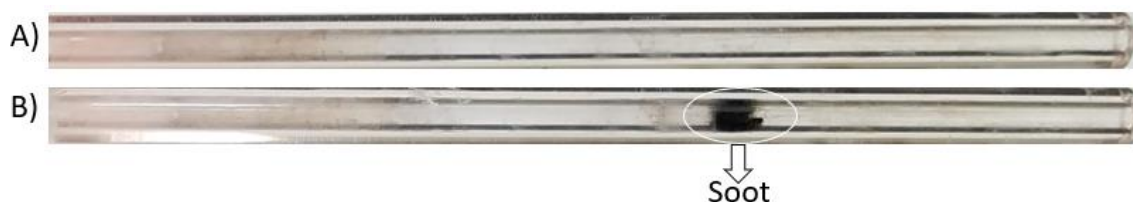
Figure 11 Reactor before(A) and after (B) combustion at a critical sooting equivalence ratio.
