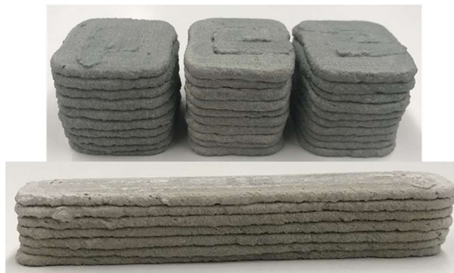
Figure 7-13: The printed mortar cubes and beam prepared for mechanical tests.
