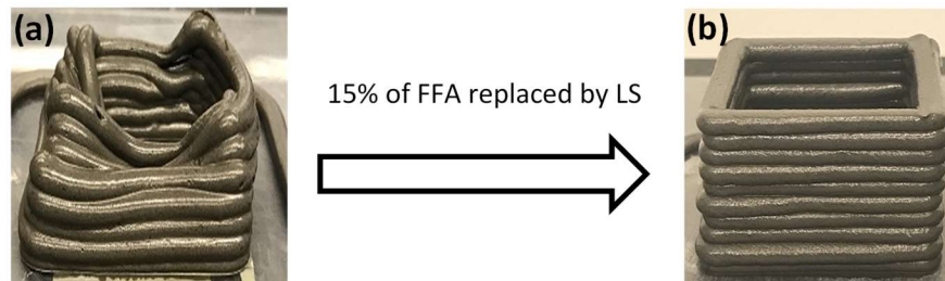
Figure 5-2: Hollow cube geometry printed using fly ash-based binders activated using 5% NaOH: (a) 100% class F fly ash paste ( l/b=0.25 ), showing shape instability, and (b) improvement in printability and buildability when 15% fine limestone is incorporated into the paste ( l/b=0.27 ).
