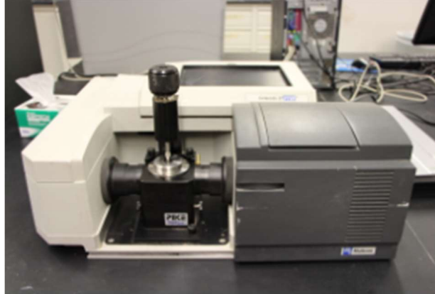
Figure 2-17: ATR Mattson Genesis FTIR spectroscope.
