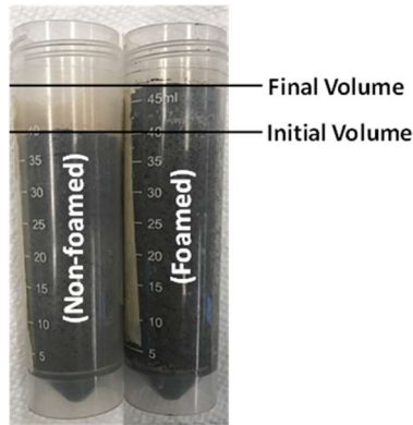
Figure 4-2: Illustration of the volume increase due to CO 2 release when the carbonate activated fly ash samples are heat cured at 100°C.
