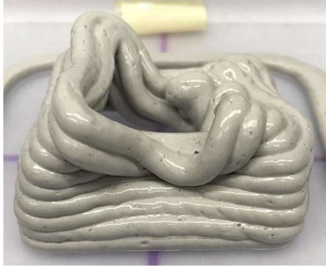
Figure 7-2: Hollow shape geometry (50 x 50 x 30 mm) printed after mixing the paste continuously for 30 min, showing shape instability.
