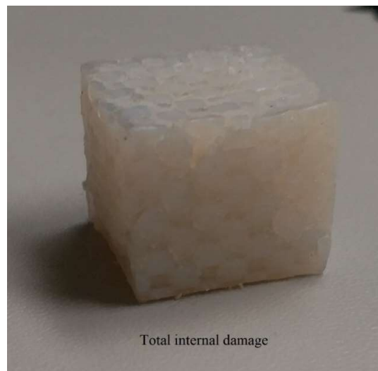
Fig 4.3: FCC structures after testing
