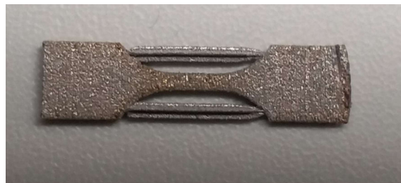
Fig 6.3: 3D printed Stainless Steel 316L alloy sample
