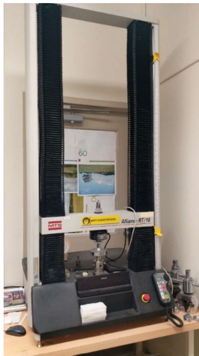
Fig 2.4: MTS Machine (Electromechanical Loading system) used for testing
