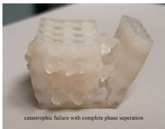
Fig 4.4: SC structures after testing
