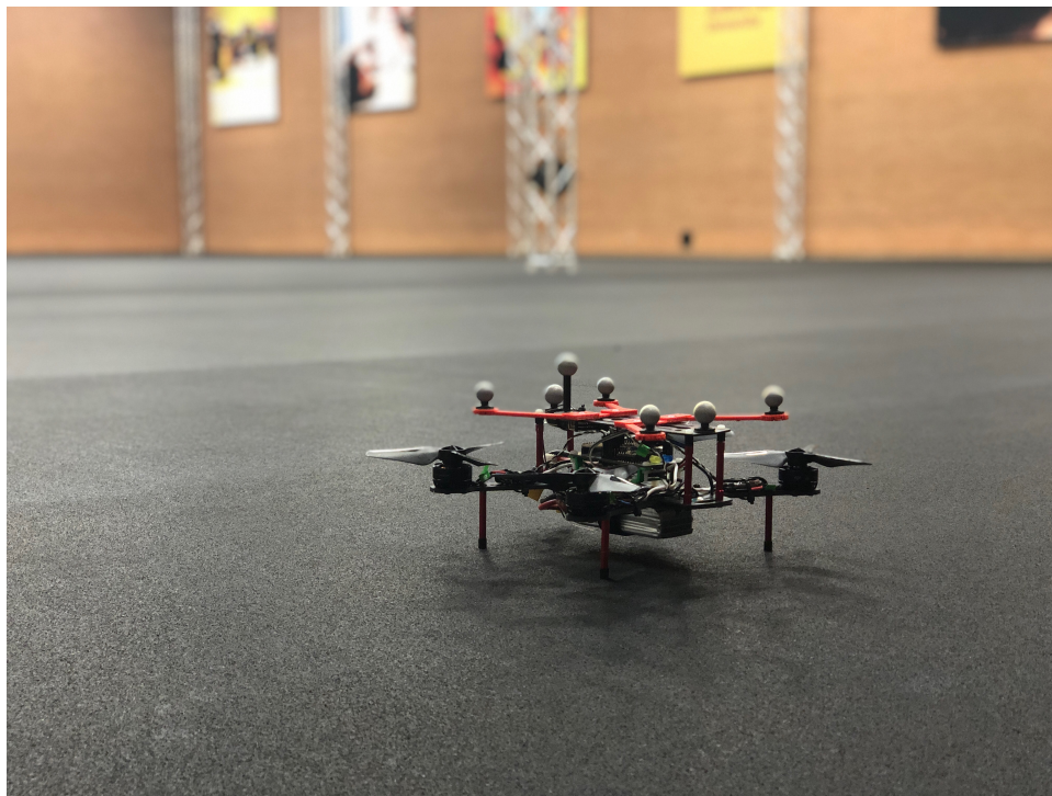
Figure 2.2: Quadrotor with Optitrack Motion Markers in ASU Drone Studio
