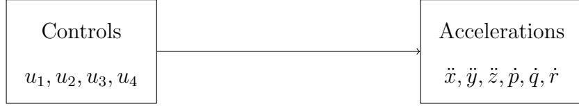
Figure 5.2: Block Diagram from Controls to Accelerations
