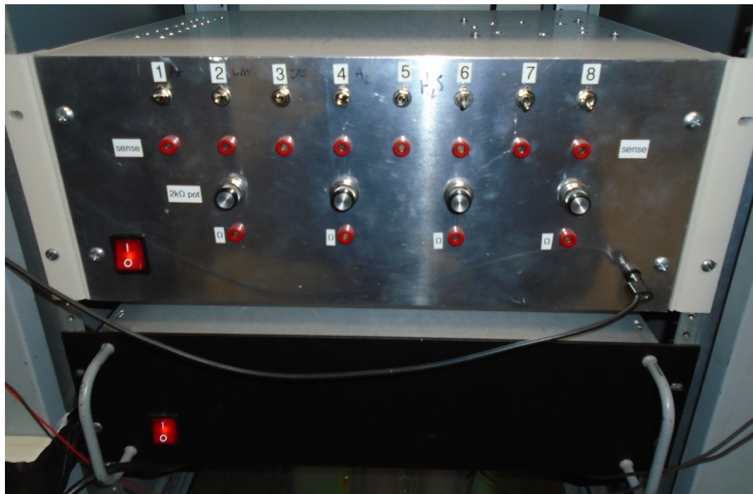
Figure 4.5: Photograph of the two instrument boxes designed and created for the automation of the growth process. The top box is the MFC control box, which directs all input and output communication between the NI USB600-1 interface and the MFCs. It also houses the power supplies and voltage dividers required by the MFCs. The row of switches at the top are in place to activate/deactivate each MFC. The red banana plugs below the switches allow the sense to be measured at any time. The four knobs below these control the division of the voltage and the final row of red plugs allow the resistance of the potentiometer to be measured. The black box underneath houses the array of solid state relays for control of the solenoid valves, and consequently control of the pneumatic valves.
