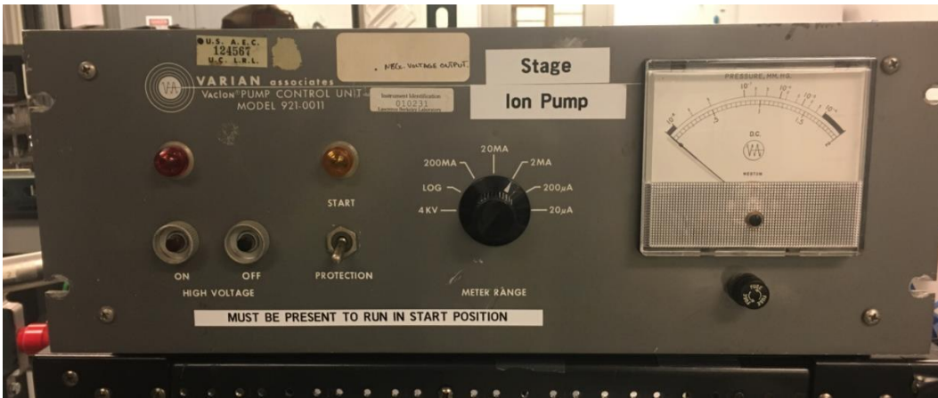
Figure 48: Ion pump power supply/control unit
