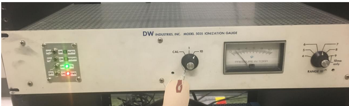
Figure 49: Ion gauge power supply/control unit
