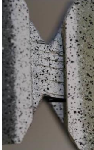
Fig. 38. Typical Failure Pattern of the Modified 1-2 Plane Shear Test Iosipescu Specimen
