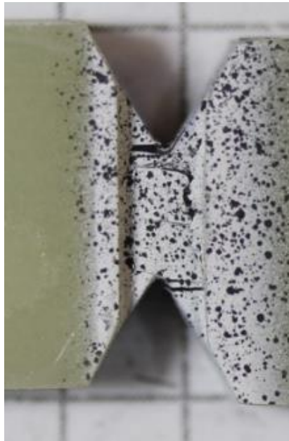
Fig. 64. Uncoupled 1-2 Plane Shear Specimen after Testing
