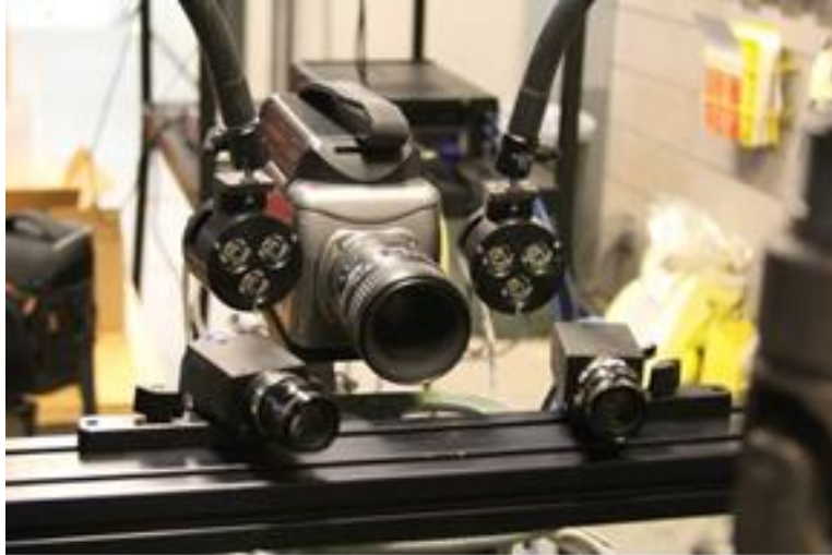
Fig. 8. Equipment Used to Capture Images During Experimental Procedures Showing Two DIC Cameras, One High Speed Camera, and Two LED Lamps
