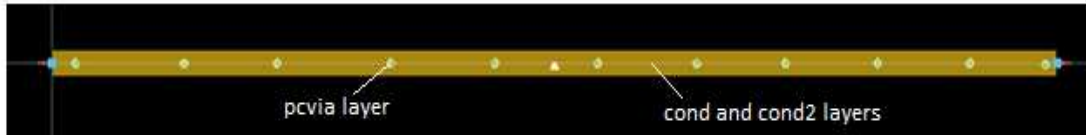
Figure 17 – Top View of the Transmission Line in ADS Momentum with Conductor and Via Layers
