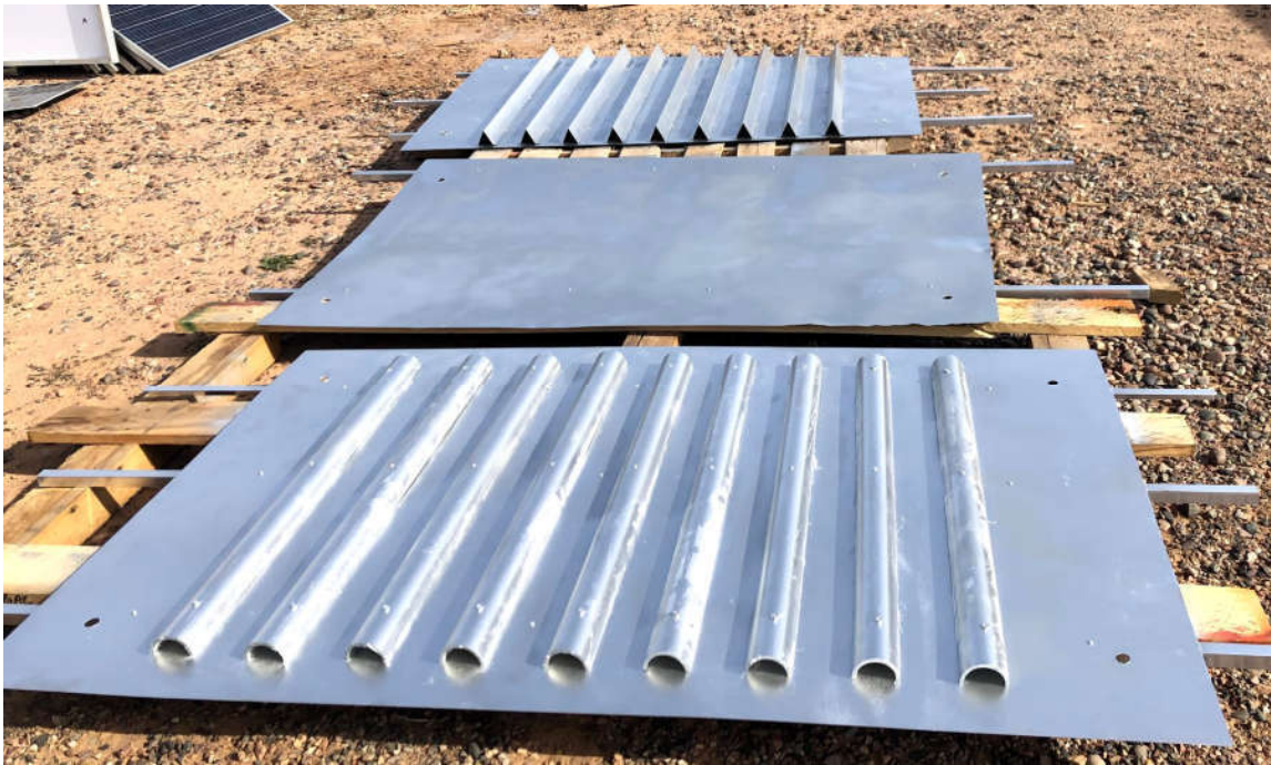
Figure 23; Profiles of reflectors utilized
