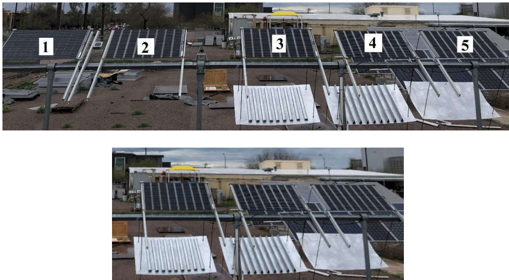
Figure 19: Test Setup with (1) 60-cell benchmark module with natural ground reflection, (2) 48-cell benchmark module with natural ground reflection, (3) 48-cell module with inverted-U reflector, (4) 48-cell module with inverted-V reflector, and (5) 48-cell module with flat reflector
