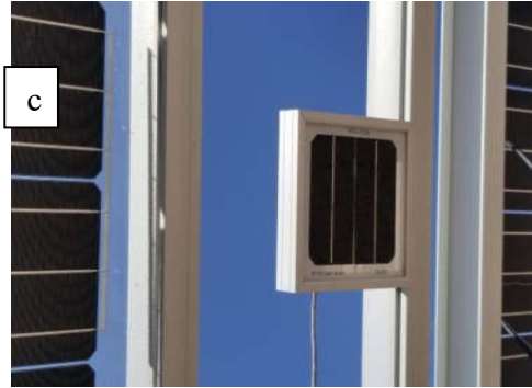
Figure 21: Mounting of reference cell; In(a) fully mounted double-faced reference cell (b) front facing reference cell (c) rear facing reference cell.
