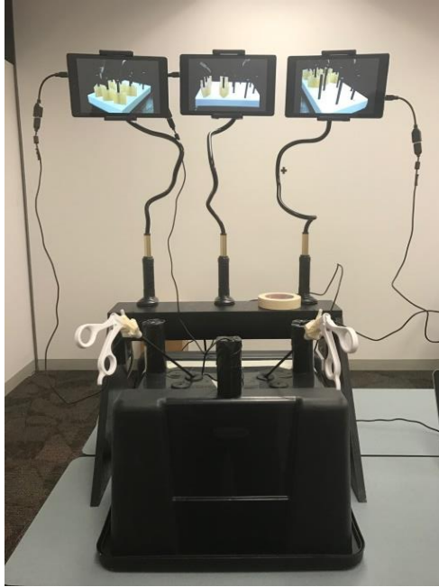
Figure 3: Constructed Laparoscopic Training Box
