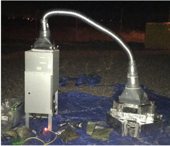
Figure 6: Burn experiment setup. Foliage was burned within the fuel bed (detailed in Figure 7), resulting combustion particles were drawn through the aluminum ductwork via the VFC sampler, and impacted clean cellulose filters at the sampling stage (Figure 8). Equipment was assembled upon a tarp to decrease soil entrainment during experiments.
