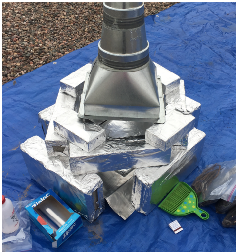
Figure 7: Contained fuel bed. Per fire marshal requirements, each burn was surrounded by aluminum foil-covered concrete blocks. To prevent tarp melting, the fuel bed consisted of an aluminum foil-covered ceramic floor tile on top of a 50 x 50 x 0.3 cm aluminum sheet and aluminum foil-covered ceramic blocks. The material for each burn was placed on top of a fresh piece of aluminum foil to prevent cross-contamination between samples and to facilitate the collection of post-burn ash.
