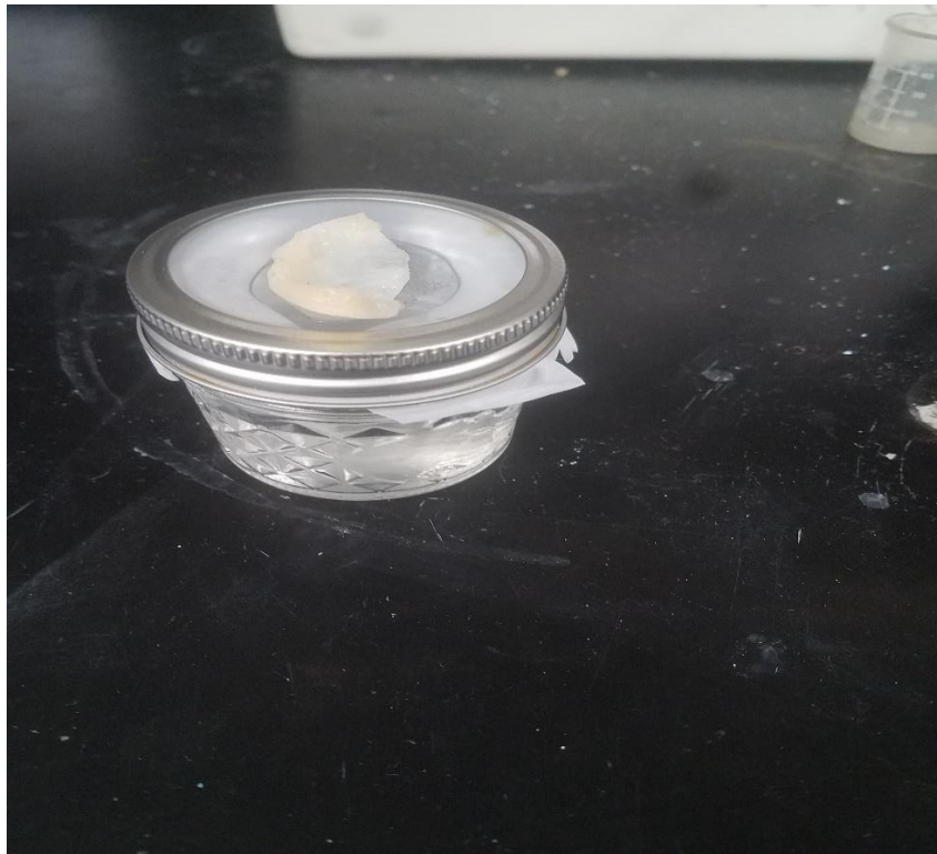
Figure 11: glass jar used as homemade FO cell module under testing. NIPAM-SA sample atop CTA membrane swelled to 5.0809g after a 48hr period, from a dry weight of 0.9103g
