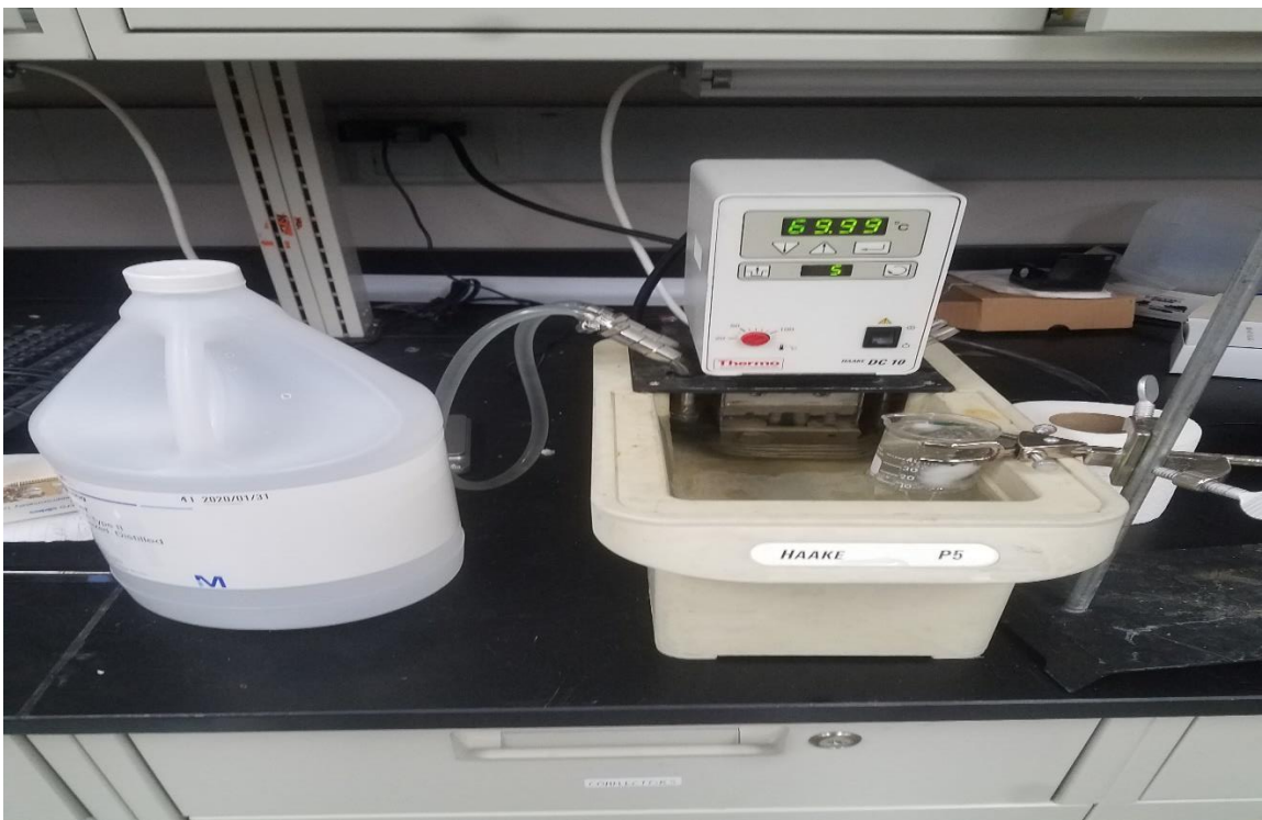
Figure 8; Experimental setup for NIPAM-SA LCST investigation.
