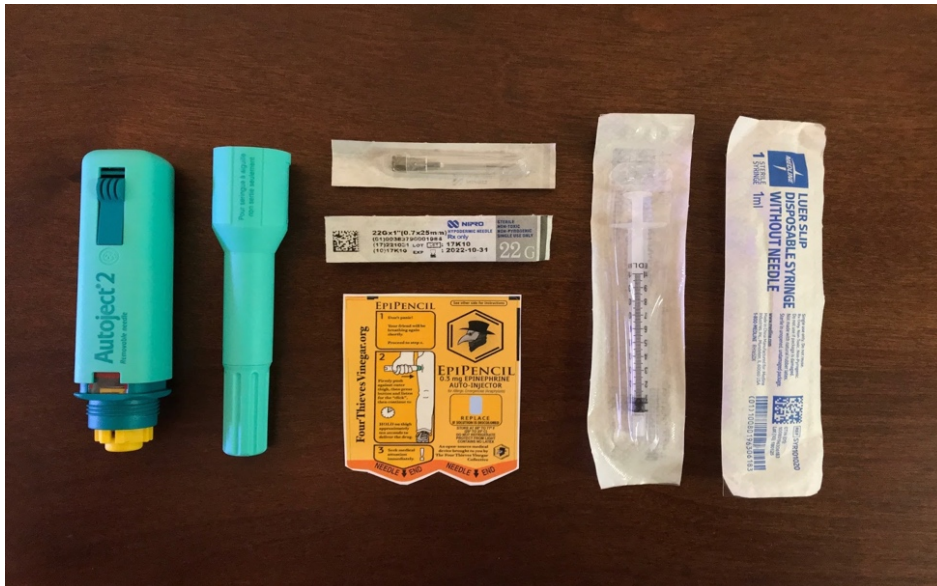
Figure 21. EpiPencil components purchased from the parts list in Table 1. Image courtesy of Matt Donovan
