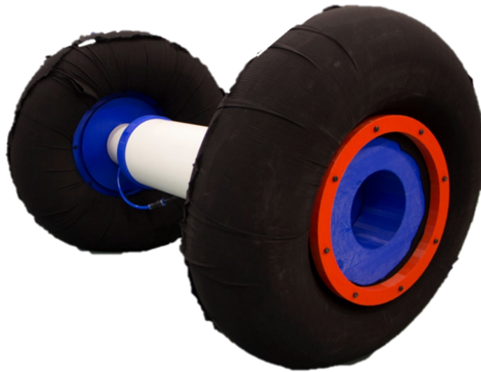
Figure 4.1: This design works in a pipeline with an inner diameter of 24 inches.
