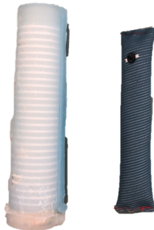
Figure 1.3: This image shows two commonly used soft robotic actuators; silicone-based on the left side and fabric-based on the right. Both of these actuators change their radial lengths when inflated.
