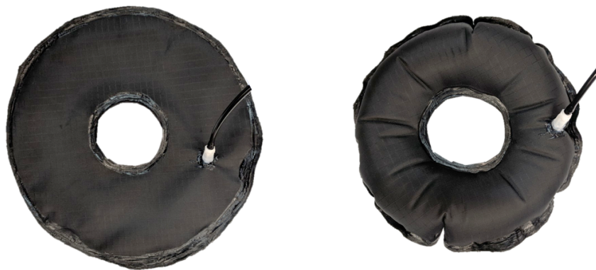
Figure 3.2: The first set of toroidal soft air actuators are shown in both a deflated and inflated state, from left to right respectively.
