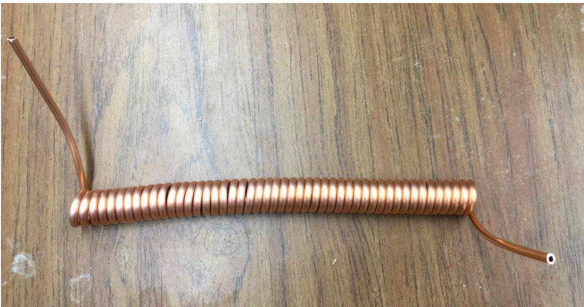
Figure 6: Copper coil as inner tube for exchanger
