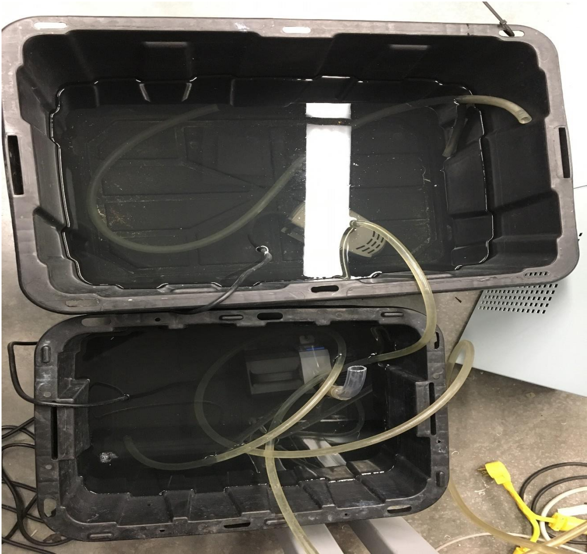
Figure 14: Cold water reservoir and return
