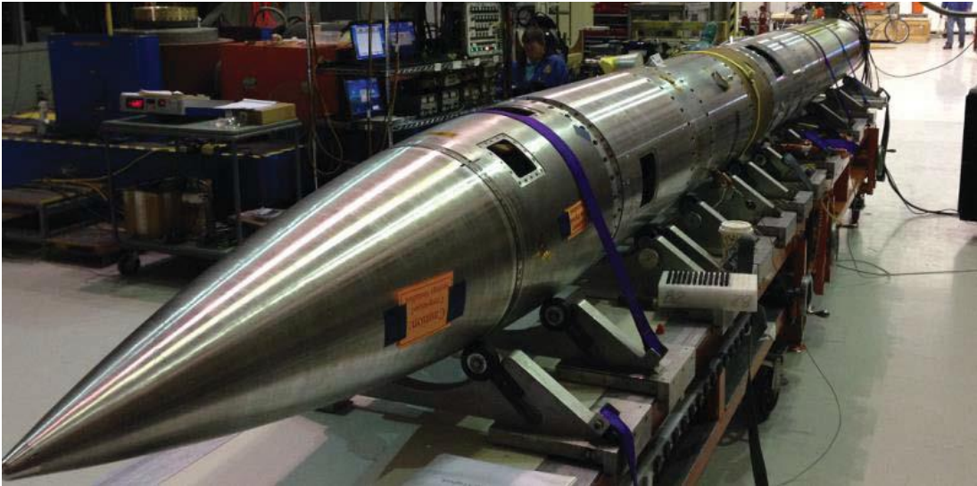
Figure 29. CHES Structure Ready for Attachment to Black Brant IX Rocket
