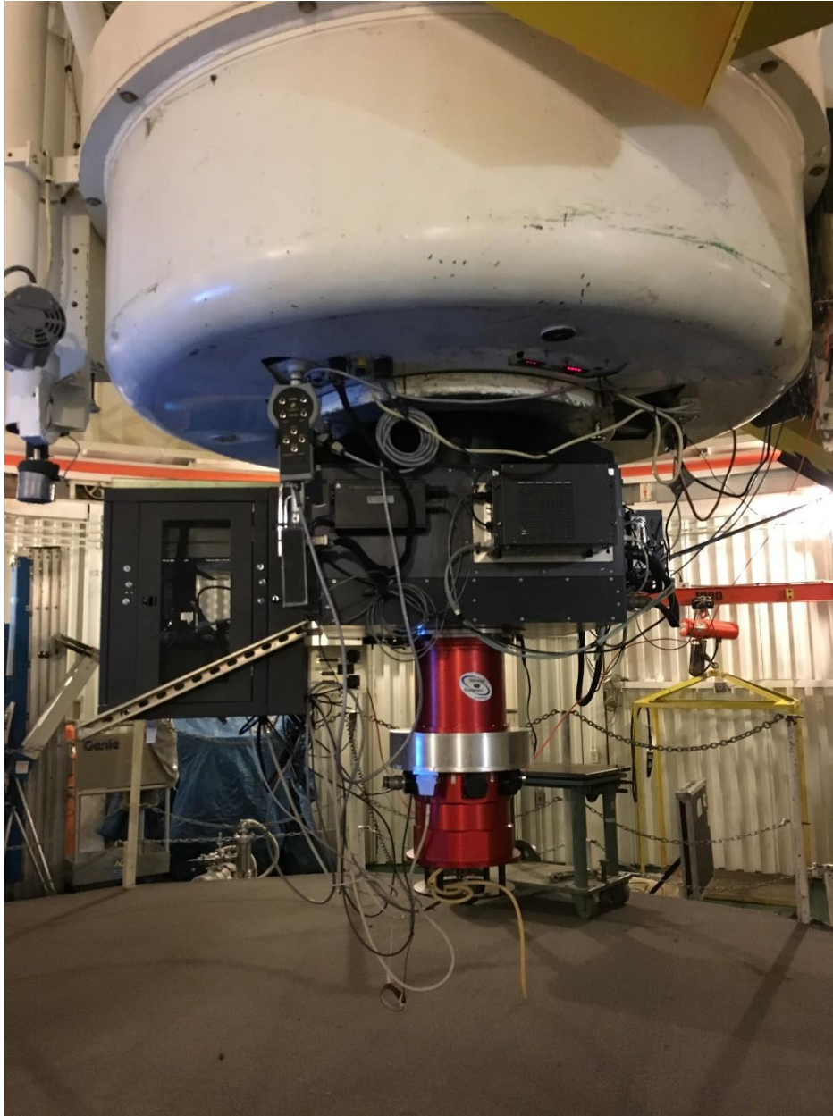
Figure 61. HERESY and Steel Instrumentation Box Mounted on Kuiper Telescope The HERESY instrumentation mounted onto the back plane of the Kuiper 61” telescope while in the ‘stowed’ position.
