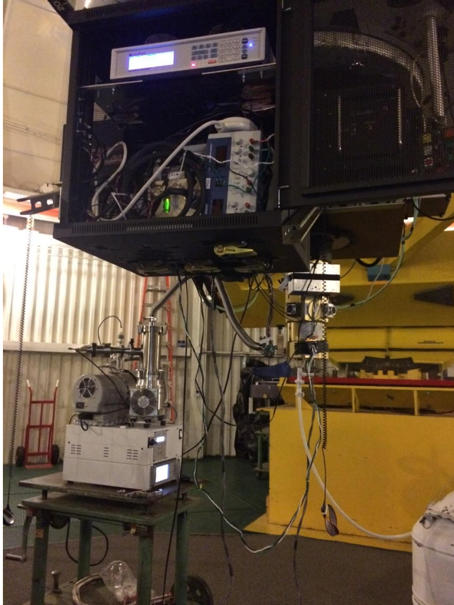
Figure 42. JPL AR-Coated CCD and associated electronics on the Kuiper 61" Telescope
