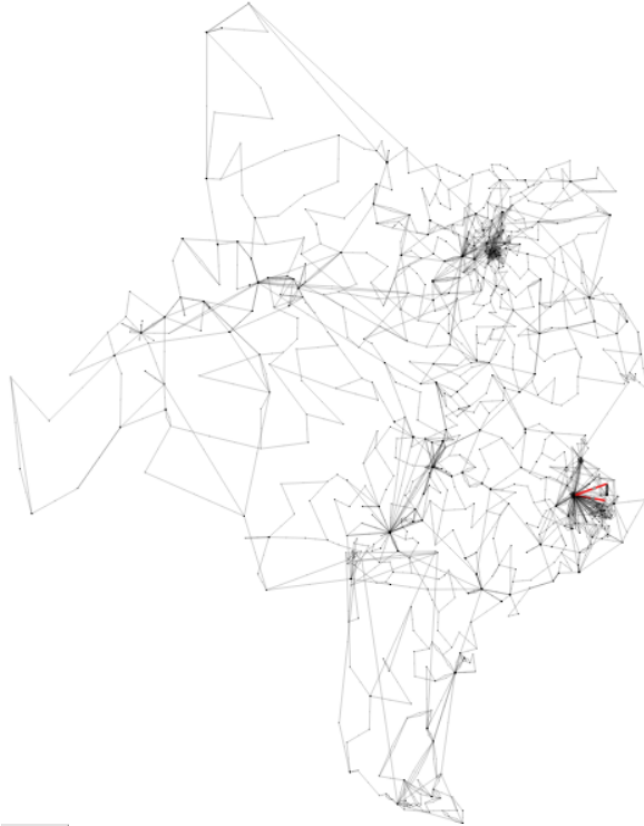
Figure 2.11: ACTIVSg (Texas synthetic) system network graph. The red branches are the branches with the bad data
