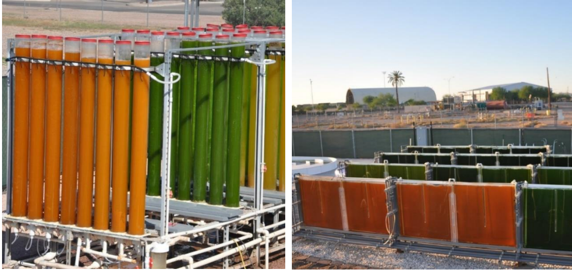
Figure 1. 8: Acrylic column photobioreactors producing Scenedesmus acutus on Arizona Center for Algae Technology and Innovation (AzCATI) field site on Arizona State University Polytechnic campus in Mesa, AZ. Photo credit: M. Villaseñor, AzCATI.
