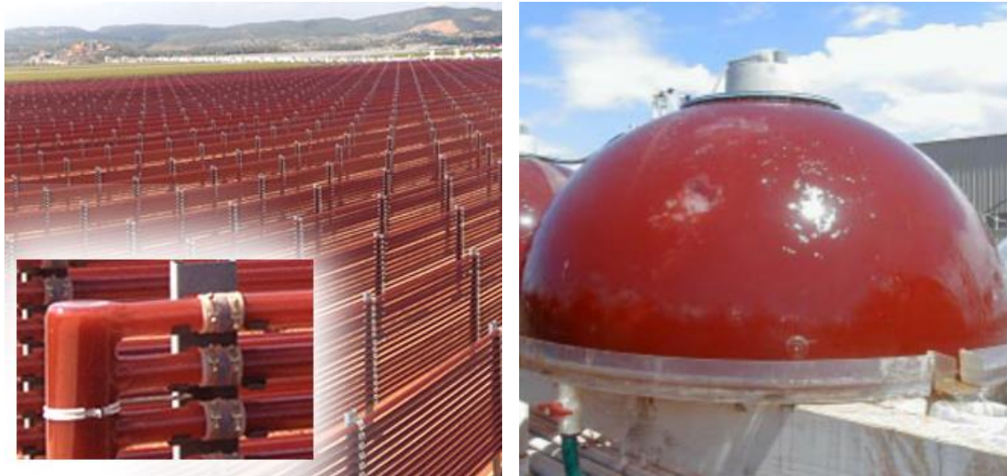
Figure 1. 10: Glass tubular photobioreactors (left) growing Haematococcus sp. for astaxanthin production in Beijing Ginkgo Group's production facility in China. This is one of the world's largest tubular systems covering 80 acres and producing 2 tons pure astaxanthin per year (BGG 2018).
