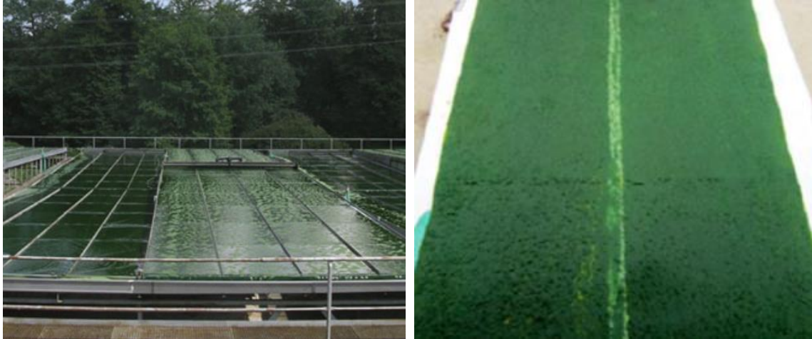
Figure 2. 1: Attached vertical biofilm reactor (right) culturing Spirulina sp. with yields of 60 \text{ gm}^{-2}\text{day}^{-1} (Zhang et al. 2015)
