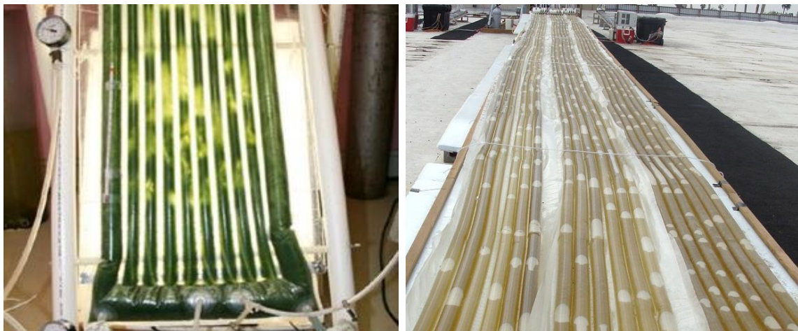
Figure 2. 3: Low-cost horizontal thin film plastic bag (right) for high-density algal growth (Photo credit: Photon 8, Inc.).
