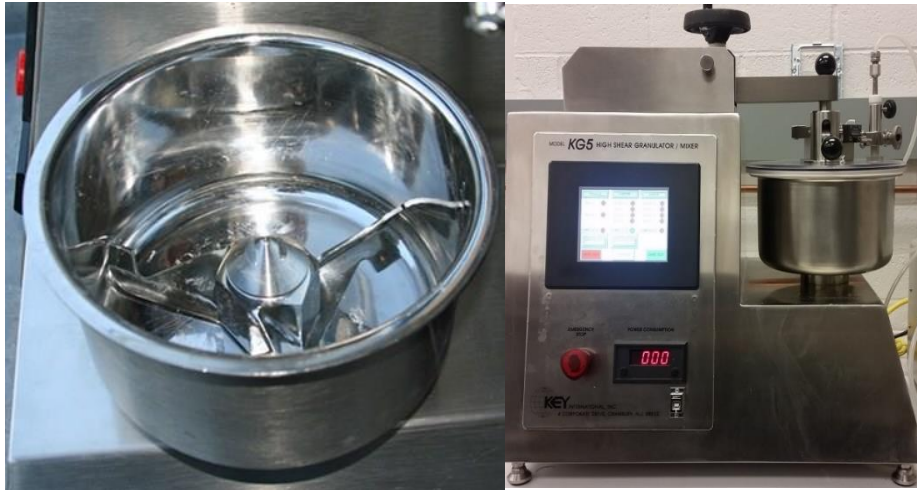
Figure 3. The container and impellor (left) for the KG5 High Shear Granulator (right).
