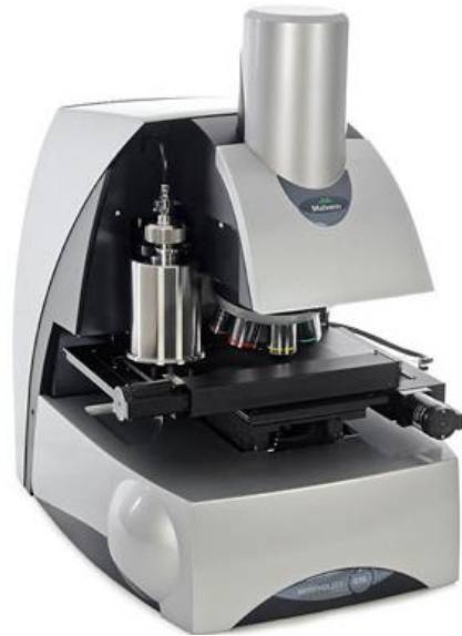
Figure 6. Malvern Morphologi G3, used to identify shape factors for 120% L/S trials in Experiment 3.
