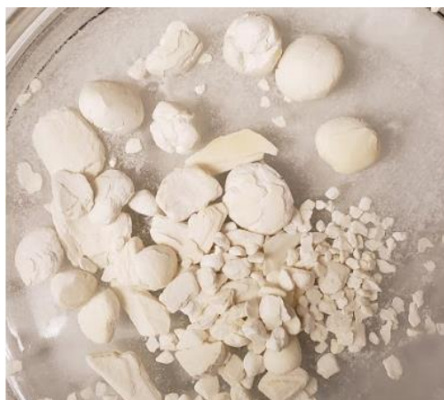
Figure 5. Microcrystalline Cellulose (MCC) and water combinations larger than 4 mm taken from an experiment trial (2/18/19) that consisted of a 120% L/S ratio, high drop height, and large drop size.
