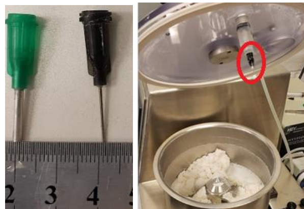
Figure 7. On the left, the large (2 mm) and small (0.2 mm) syringe nozzles, and on the right, the modified syringe apparatus attached to the spray nozzle.
