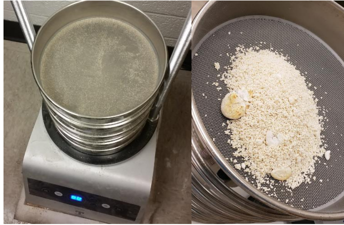
Figure 4. The electric sieve shaker (left), and example 12” diameter sieves (right) used to separate dried granules by size.
