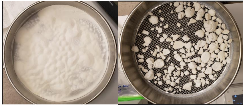
Figure 17. The remaining ungranulated powder (left) and granules larger than 3 mm (right) of the 80% L/S ratio low drop height large drop size trial in Experiment 3.
