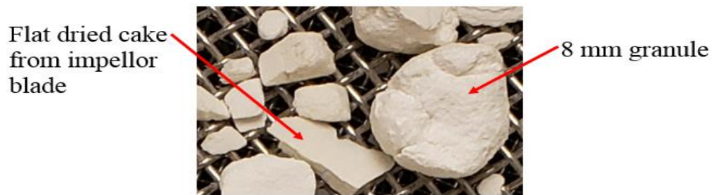
Figure 11. Examples of two combinations of MCC and water greater than 4 mm: dried cake from the impellor blade (left) and a large irregular granule (right).
