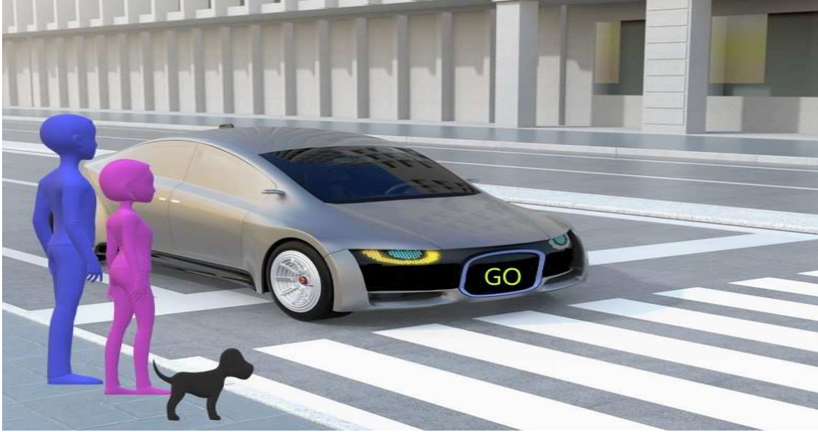
Figure 1. An example of an image used in the survey. This image is using the word “go” to indicate pedestrians can safely navigate the intersection.
