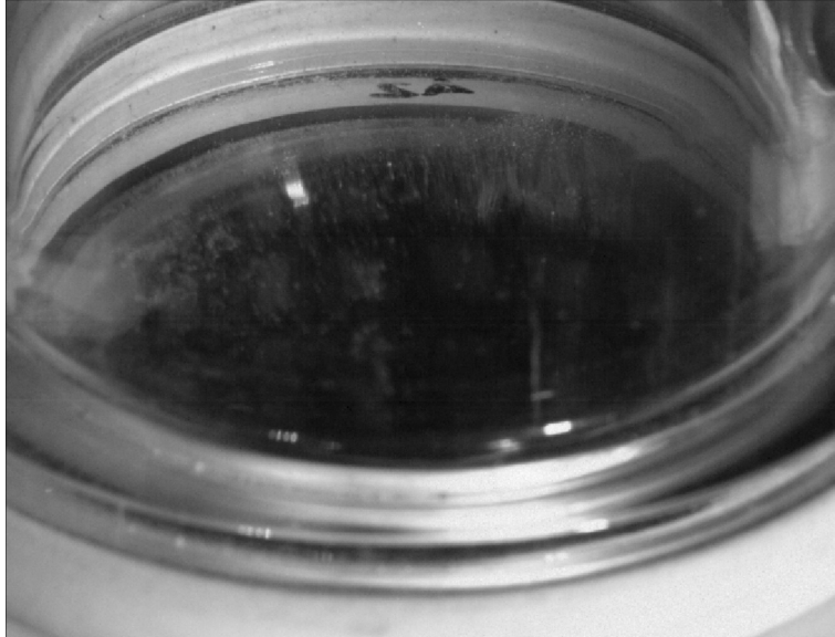
Figure 25: Shown Is an Image Taken a Few Ten-thousandths of a Second after the Image Shown in Figure 24. Visible in the Upper Right Portion of the Diaphragm (Approximately 1 O'clock in Clock Position), Is the Initial Tear That Occurs as the Nichrome Melts Through the Polypropylene. Several Particles Are Visible Flying Upward Away from That Region as Evidence That Gas Flow Is Present and the Diaphragm Is about to Rupture Completely—Called the Large Rupture Event.
