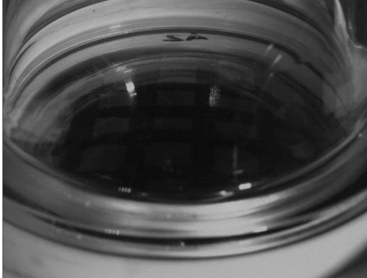
Figure 24: Shown Is a Closeup of the Diaphragm. The Top of the Diaphragm Has Been Marked with a Dark Grid to Show the Dramatic Flexion and to Better Identify the Location of the Diaphragm, as It Is Difficult to See the Clear Polypropylene Material.
