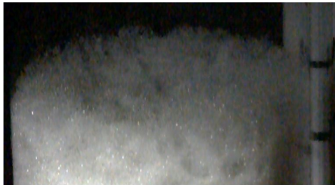
Figure 33: Shown Is a Time Progression of the Particle Bed Interface. Note That the Edges of the Particle Bed Rise Earlier than the Interior of the Interface. The Starred times Signify the Time from When Any Motion in the Particle Bed Is Seen at All to When the Associated Image Was Taken.
