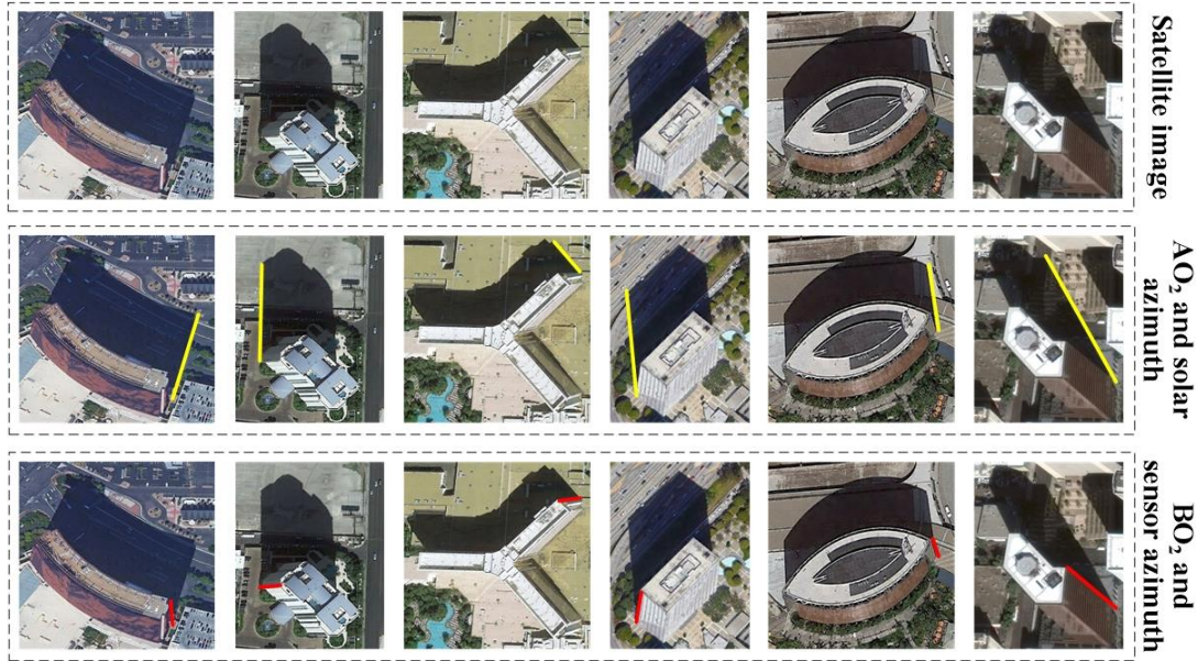
Figure 9. Illustration of buildings visualized by the VHR image, the line segment for accessing the length of AO_2 and the sensor azimuth ( \theta_1 ) shown in Figure 4(C), and the length of BO_2 and the solar azimuth ( \theta_2 ) shown in Figure 4(C).
