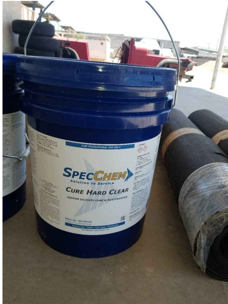
Picture 3.7: Concrete Cure Used for Test Slabs in Phoenix Slabs
