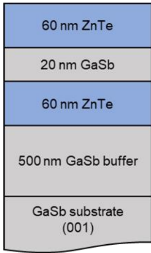
Fig. 28: Schematic growth structure and XRD pattern for the GaSb/ZnTe quantum well sample.
