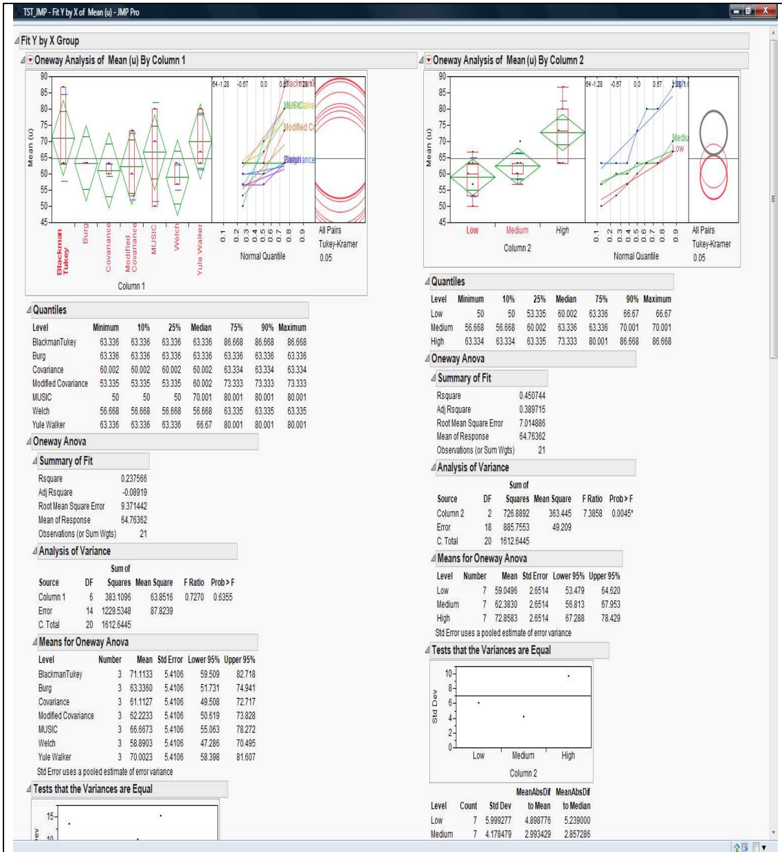
Figure 89. ANOVA analysis of output results (Plot 1: (L) Algorithm vs Mean & Plot 2: (R) Resolution vs Mean)
