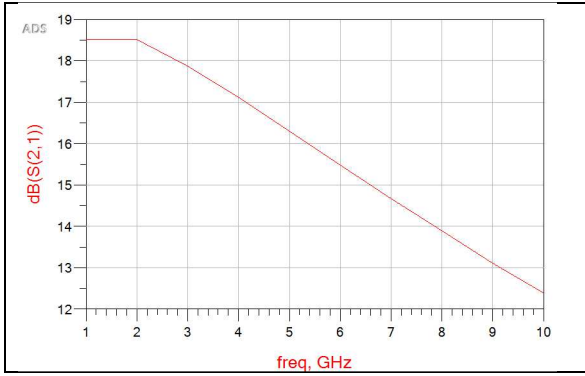
Figure 45 Broadband P-HEMT LNA Performance Curve
