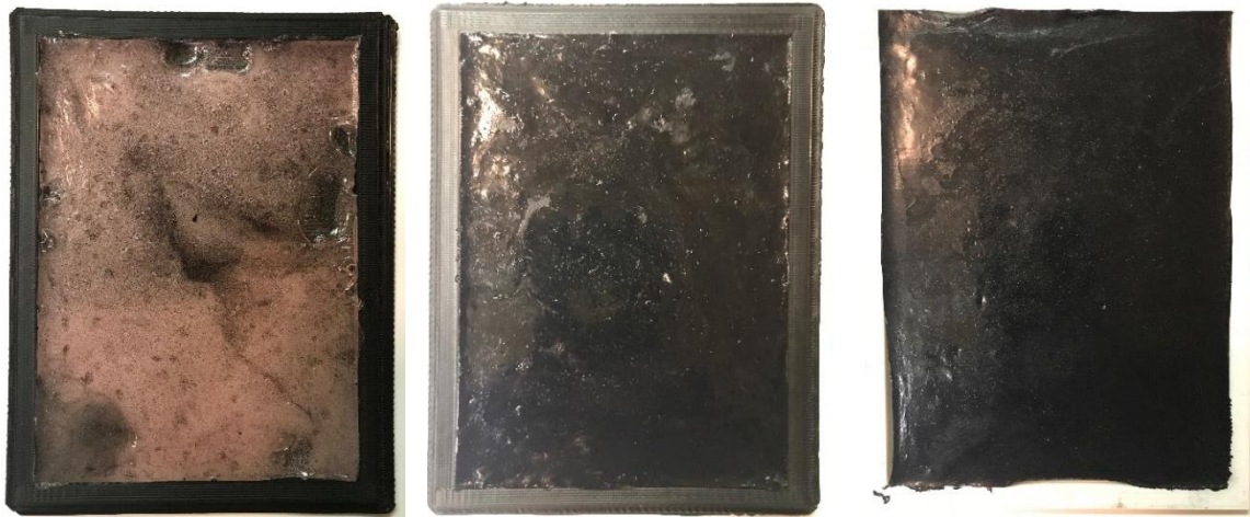
Figure 20. (Left) The Unprepared Non-Additive In-Mold Sample Flat. (Middle) The Unprepared 1.5% Loaded Carbon Black In-Mold Sample Flat. (Right) The Unprepared 2.3% Loaded Carbon Black In-Mold Sample Flat.
