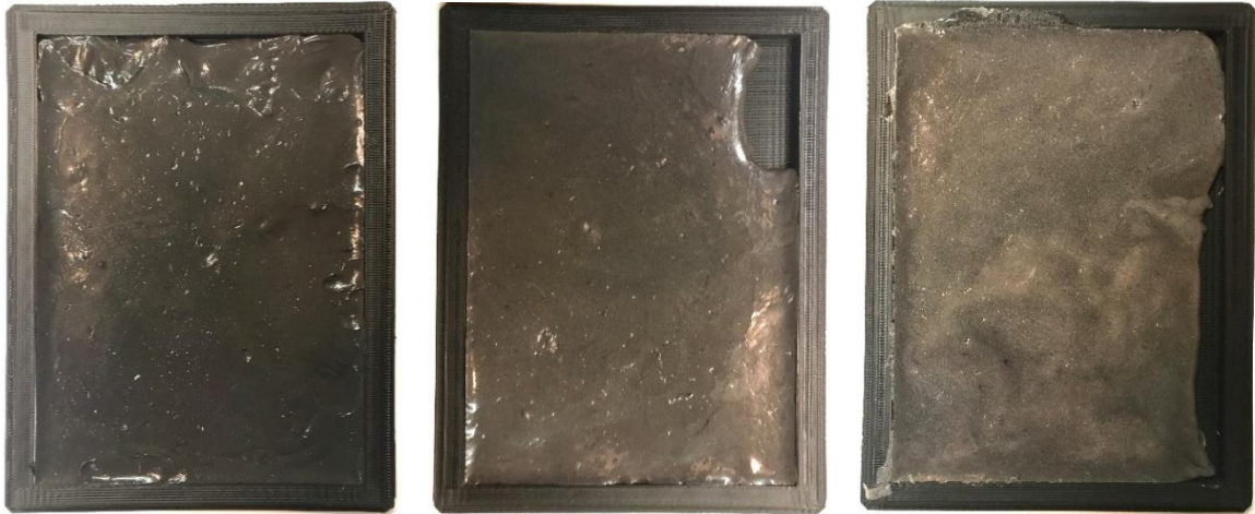
Figure 21. The Unprepared 1.5% Loaded Tungsten (Left) 1-5 Micron, (Middle) -325 Mesh, and (Right) -100 Mesh In-Mold Sample Flats.
