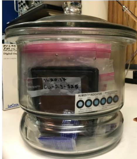
Figure 12. Testing Samples Stored in the Laboratory Desiccator.
