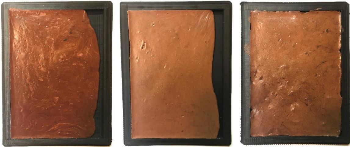
Figure 26. The Unprepared 5% Loaded Copper (Left) 1-5 Micron, (Middle) -325 Mesh, and (Right) -100 Mesh In-Mold Sample Flats.
