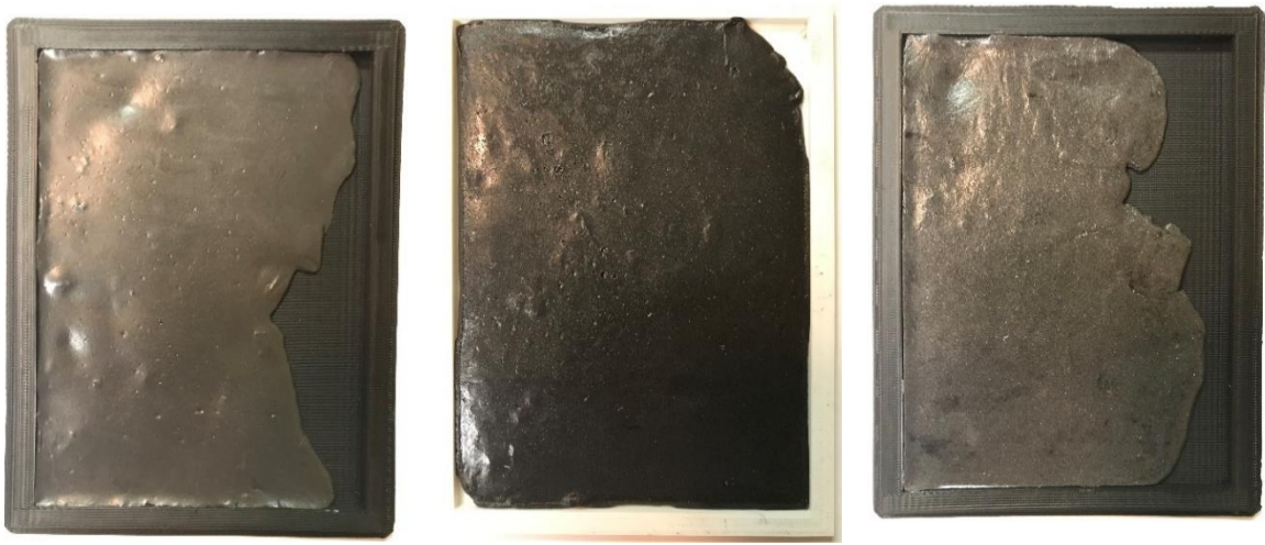
Figure 23. The Unprepared 5% Loaded Tungsten (Left) 1-5 Micron, (Middle) -325 Mesh, and (Right) -100 Mesh In-Mold Sample Flats.
