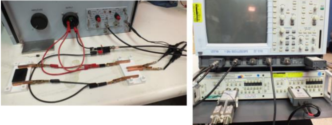
Figure 15. (Left) The Testing Apparatus Integrated into the Testing Set-up. (Right) The Oscilloscope and Differential Amplifier with Connections from the Testing Set-up.
