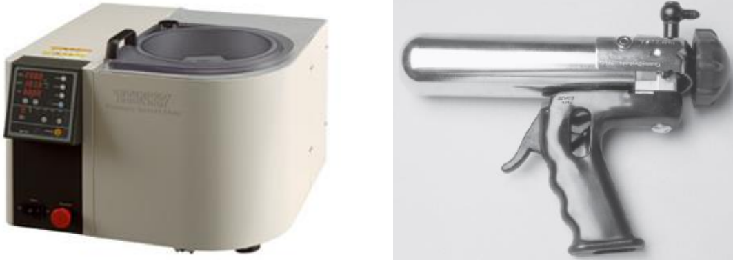
Figure 11. (Left) Thinky Mixer Used to Manufacture Test and Final Sample Formulations [41]. (Right) The Semco extruding gun used to extrude mixed propellant out of the syringes in which they were mixed.
