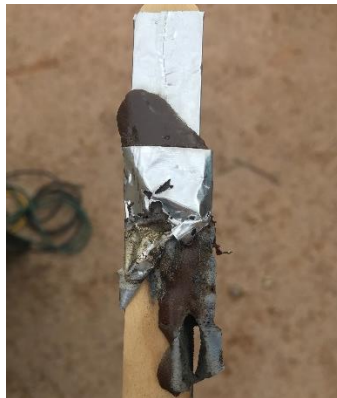
Figure 19. An Improvised Coaxial Electrode Thruster Shown After Being Pulsed Several Times.
