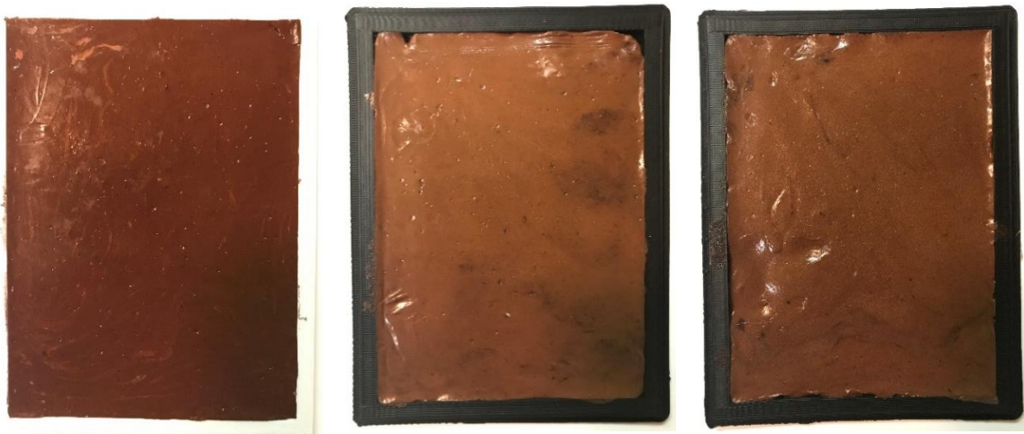
Figure 25. The Unprepared 2.3% Loaded Copper (Left) 1-5 Micron, (Middle) -325 Mesh, and (Right) -100 Mesh In-Mold Sample Flats.
