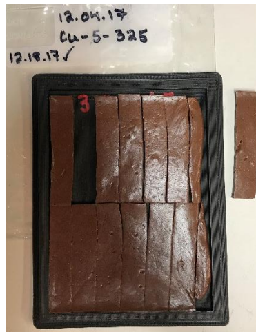
Figure 27. A Prepared Sample Flat and Storage Bag, with a Randomly Chosen Specimen Removed from Flat Mold to Display the Specimen Labeling Technique.
