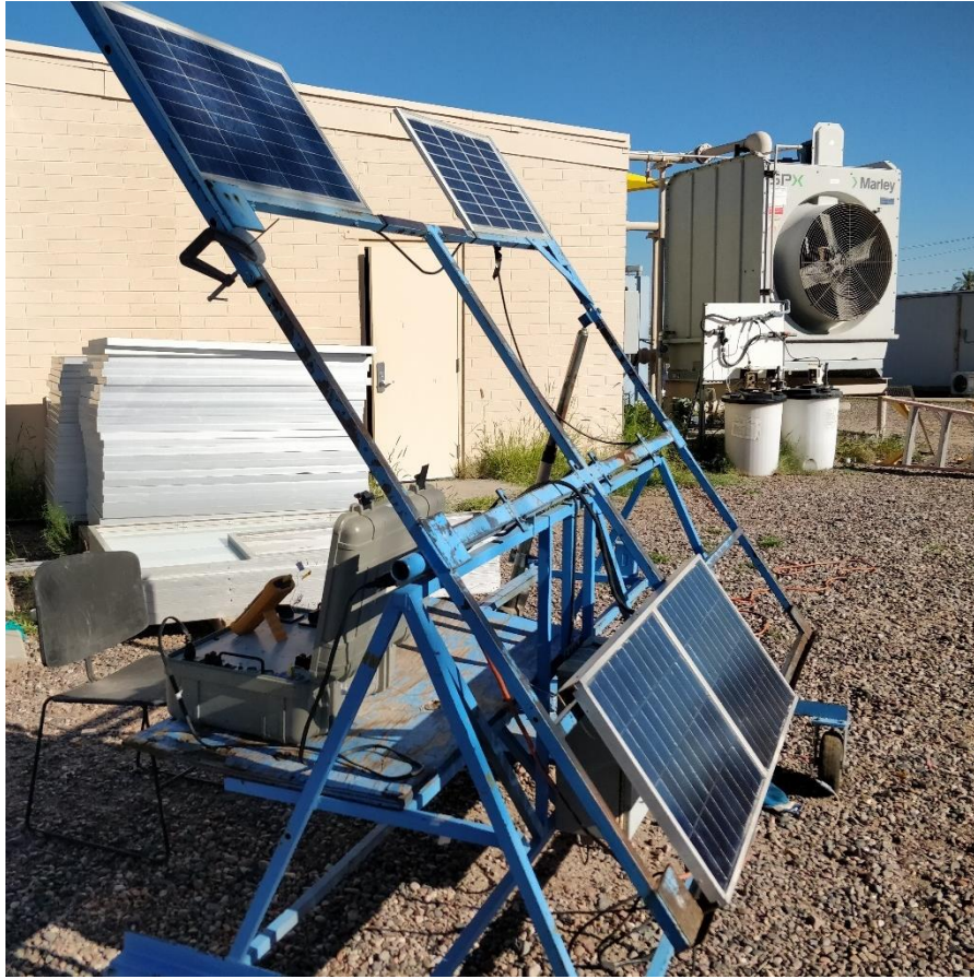
Figure 5. Outdoor IV setup with two axis tracker and PV module connected in forward bias to the curve tracer for measuring IV curves.
