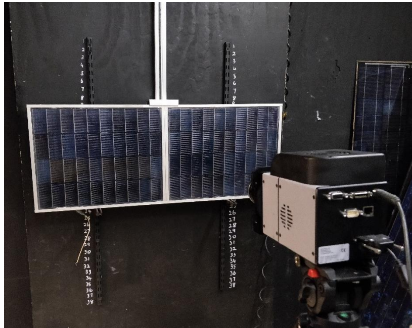
Figure 6. EL imaging setup in a dark room with camera facing the PV module.
