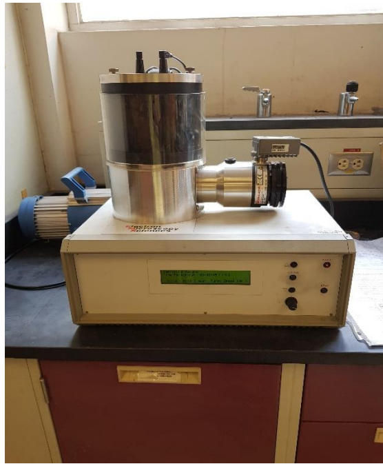
Figure 11 Carbon coating setup used to coat samples with thin carbon layer
