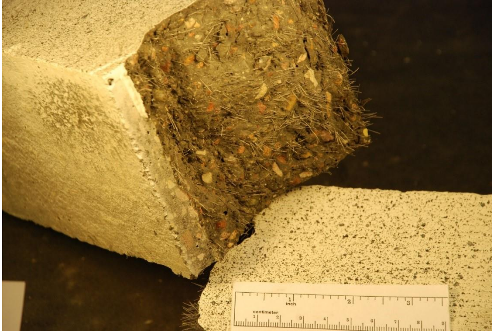
Figure A. 12. Large beams, 4" x 4" x 16" (102 mm x 102 mm x 406 mm), with 3% fiber content, after 28 days (FML_L_3_28_3PB_C_B3).
