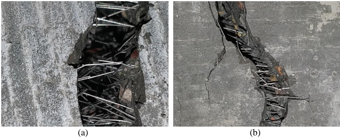
Figure 6. Bridging effect of fibers on samples with: (a) 1% fiber content; (b) 3% fiber content.
