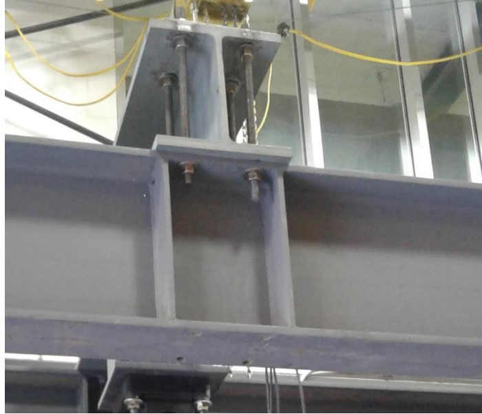
Figure A. 59. Connection of the Loading Beam (BI) to the Top Beams (BII).
