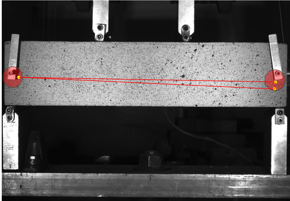
Figure 25. Three-point reference for rigid body movement of the sample.
