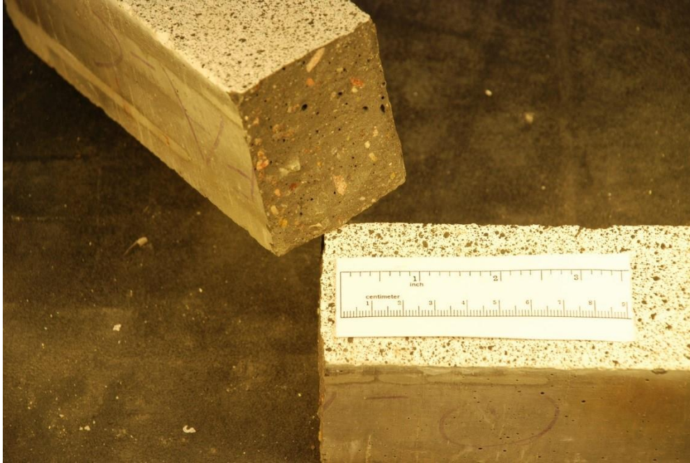
Figure A. 33. Small beams 2" x 2.5" x 14", with 1% fiber content, after 28 days (FML_S_0_28_4PB_C_B2).
