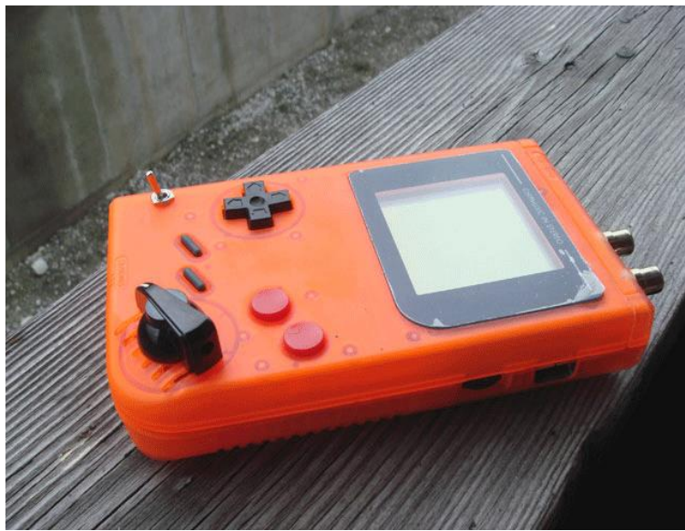
Figure 90. A DMG with a clocking switch and potentiometer, as well as two additional audio outputs. Source: chipmusic.org/forums/topic/7345/customized-gear-thread/page/5/
