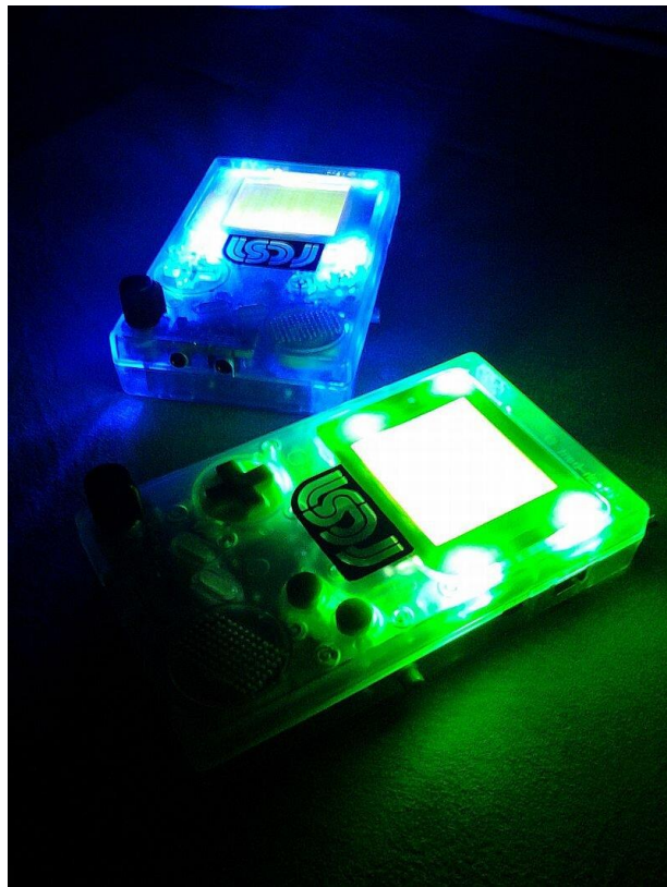
Figure 72. Two DMGs with LED mods, a clocking mod and prosound mod. Source: chipmusic.org/forums/topic/7345/customized-gear-thread/page/25/
