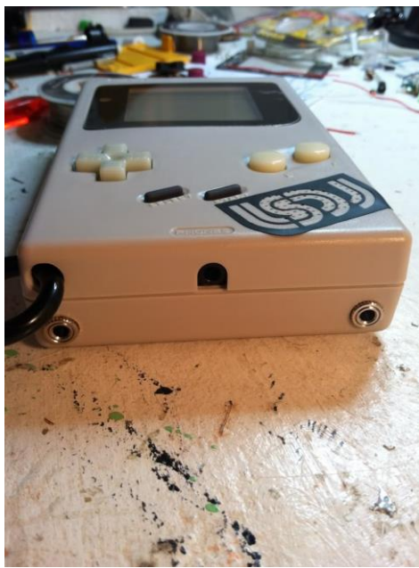
Figure 81. Adding two 1/4" audio outputs for the left and right channels. Source: chipmusic.org/forums/topic/7345/customized-gear-thread/page/5/
