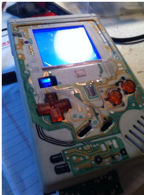
Figure 62. An example of a custom case with backlight. This “Circuit Boy” also has LEDs in the battery case (not pictured here). Source:
