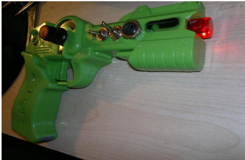
Figure 94. Adding a potentiometer (knob) to control the pitch, toggle switches to pitch down or loop, and a 1/4" audio jack to a toy gun. Source: chipmusic.org/forums/topic/14499/circuit-bent-stylophone-beatbox-circuit-bent-toy-gun/
