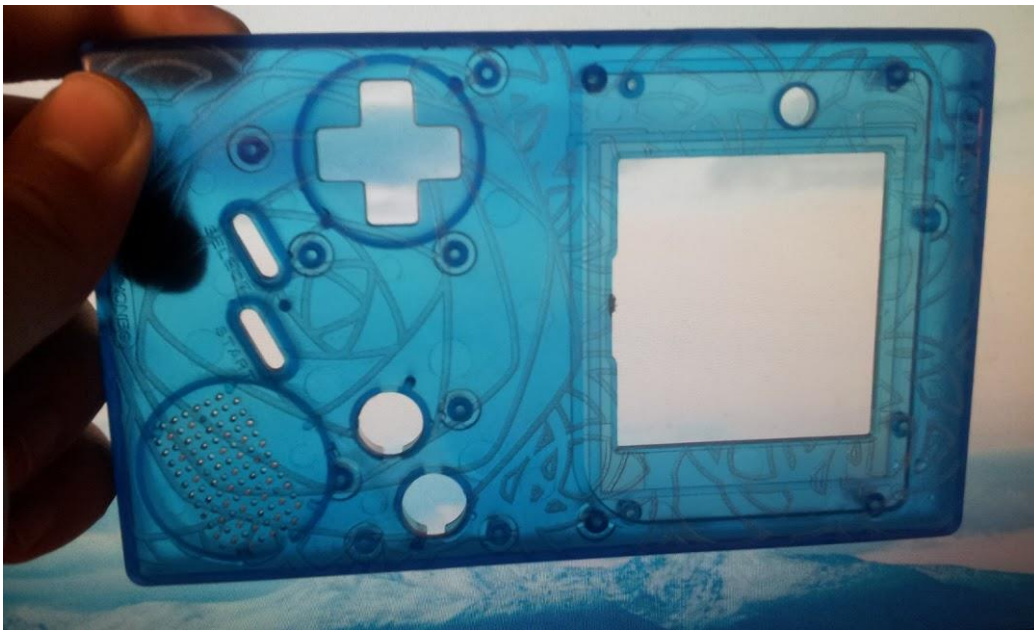
Figure 66. Laser engraving a DMG case. Source: chipmusic.org/forums/topic/12223/laser-engraving-take-two/page/4/
