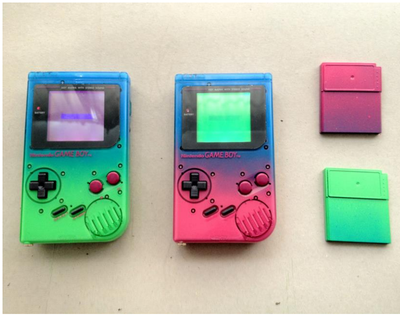
Figure 58. Two painted DMGs with prosound and backlight mods. Source: chipmusic.org/forums/topic/7345/customized-gear-thread/page/10/
