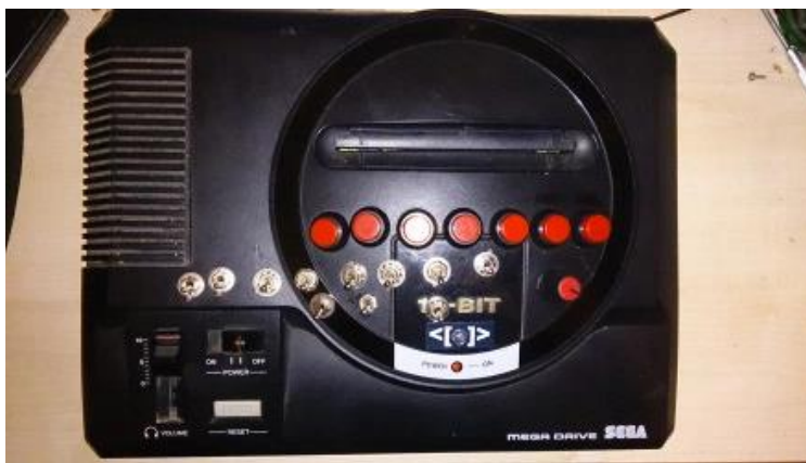
Figure 26. An example of a circuit-bent SEGA Megadrive. This member added red buttons to trigger sound glitches and switches to toggle video glitches. Source: chipmusic.org/forums/topic/14965/circuit-bent-megadrive-lotus-ii-rewire/
