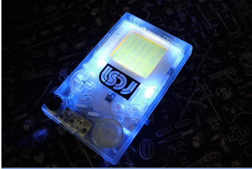
Figure 71. An example of an LED mod inside a clear DMG. Source: chipmusic.org/forums/topic/7345/customized-gear-thread/page/16/
