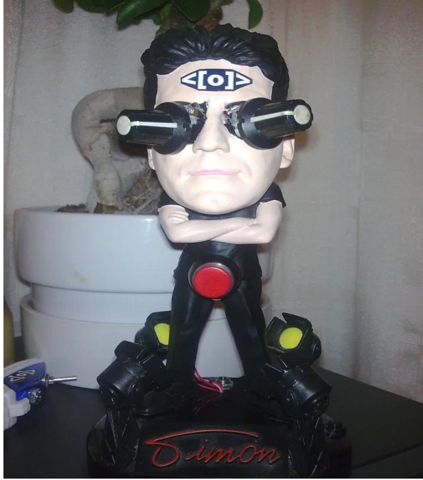
Figure 93. Adding potentiometers (knobs) and a button to a Simon Cowell talking bobble head. Source: chipmusic.org/forums/topic/15247/circuit-bent-slimeon-cowell-talking-figure/
