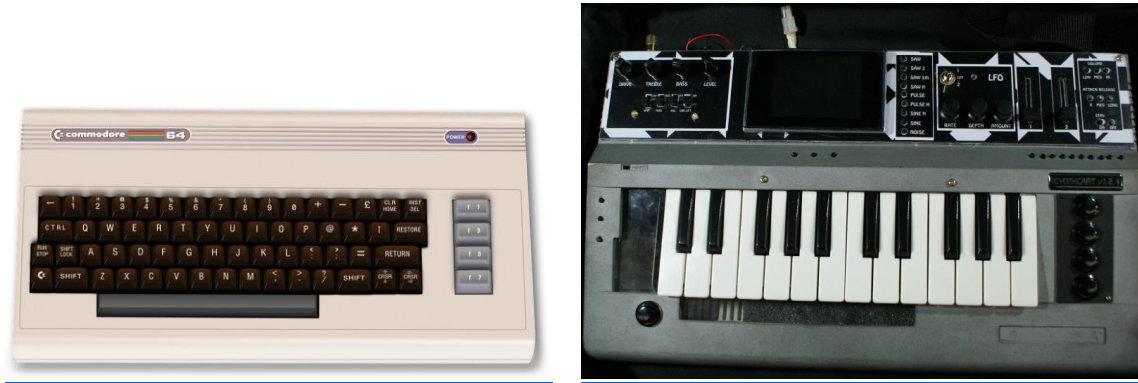
Figure 97. Repurposing a Commodore 64 keyboard (pictured left) as a MIDI keyboard with several external devices (pictured right). Left image source: pixabay.com/p-2154499/?no_redirect Right image source: chipmusic.org/forums/topic/15249/c64c-mods/page/3/
