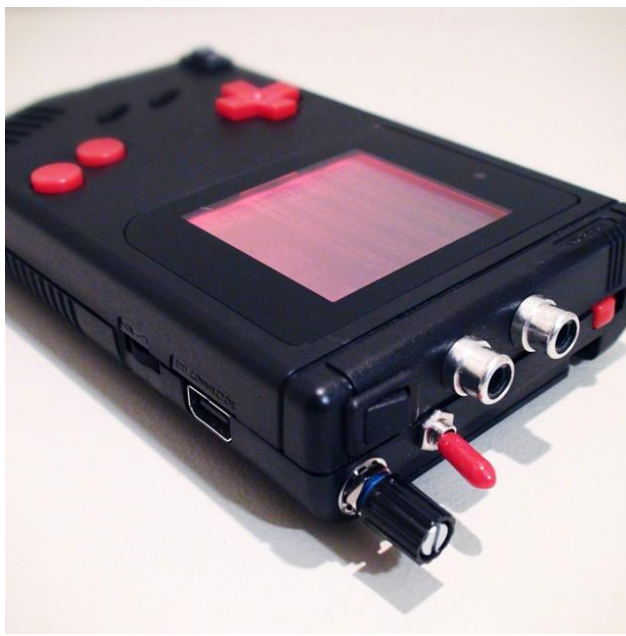
Figure 82. Adding two audio outputs and a switch/potentiometer for clocking. Source: chipmusic.org/forums/topic/7345/customized-gear-thread/page/73/
