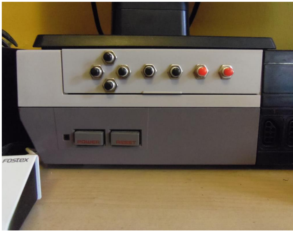
Figure 98. Adding controller buttons to the Nintendo Entertainment System's (NES) case. Source: chipmusic.org/forums/topic/4601/modified-nesmidines-with-midi-in-socket-front-panel-control/
