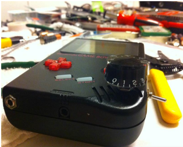
Figure 88. A DMG with a switch and potentiometer to adjust the clock speed. This mod is also known as a “pitch mod” because the clock speed affects the pitch. Source: chipmusic.org/forums/topic/7345/customized-gear-thread/page/5/
