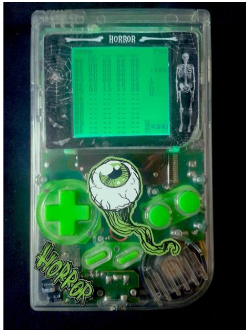
Figure 61. A DMG with modified buttons, artwork, and an inverted yellow backlight.
